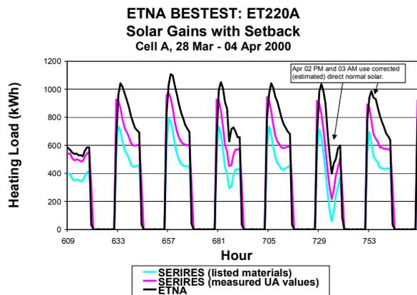
Figure 7. Simulation versus Empirical Data Results, Dynamic Thermal Diffusion With Solar Gains And Thermostat Set Back
