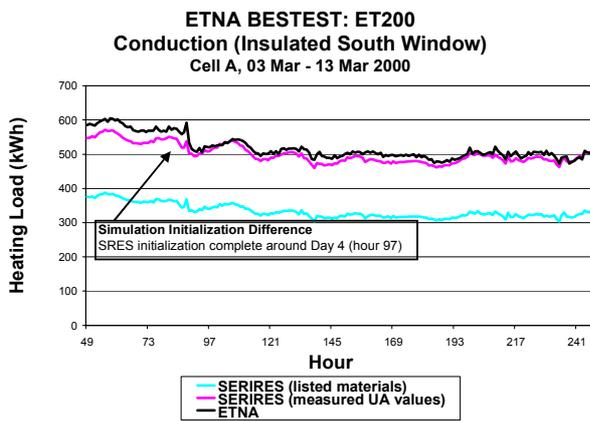
Figure 4. Simulation versus Empirical Data Results, Dynamic Thermal Diffusion Without Solar Gains
