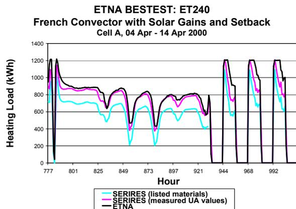
Figure 8. Simulation versus Empirical Data Results, Dynamic Thermal Diffusion Using Typical French Convector (in place of HWD) With Solar Gains And With and Without Thermostat Set Back
