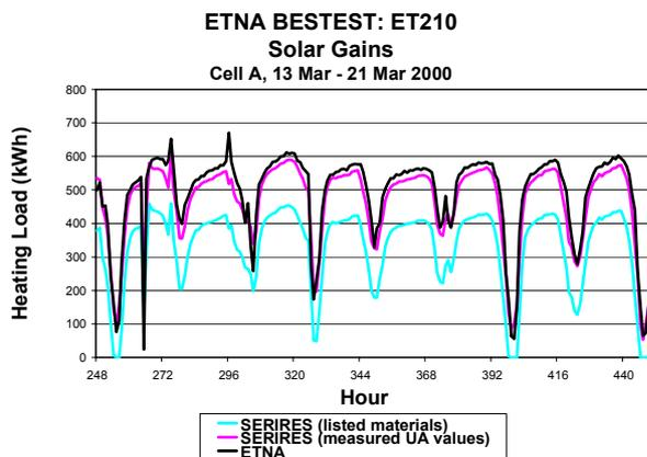
Figure 5. Simulation versus Empirical Data Results, Dynamic Thermal Diffusion With Solar Gains
