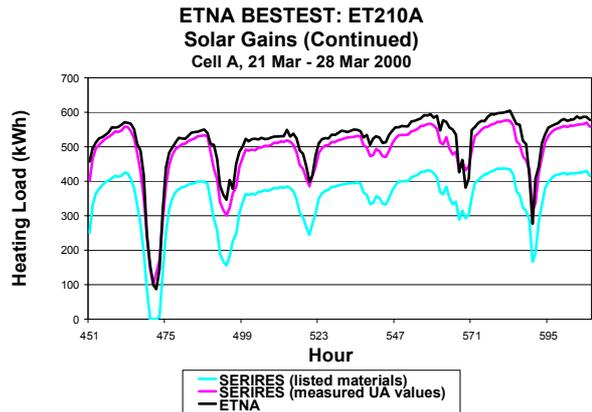
Figure 6. Simulation versus Empirical Data Results, Dynamic Thermal Diffusion With Solar Gains (ctd.)
