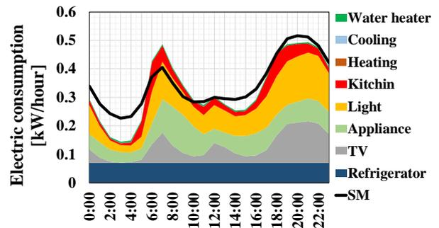
Figure 3: Average electricity consumption versus time of day after delaying bedtime by two hours
