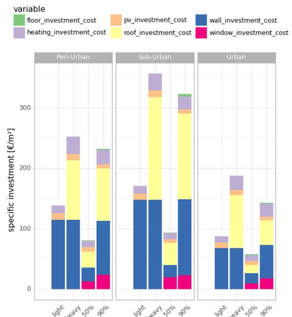
Figure 8 Breakdown of specific investment costs as € per m<sup>2</sup> floor area.
