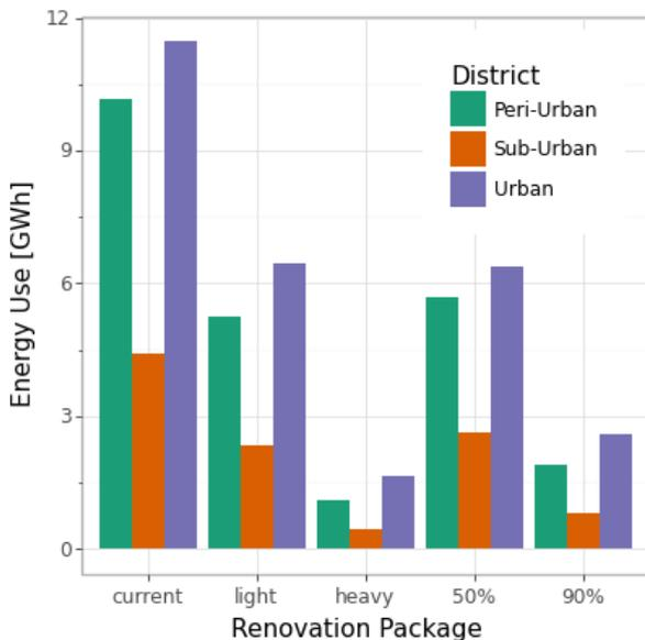
Figure 3 Total energy use as function of the renovation packages
