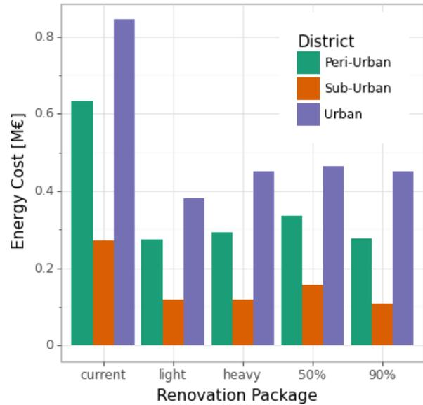
Figure 4 Total energy cost as function of the renovation packages
