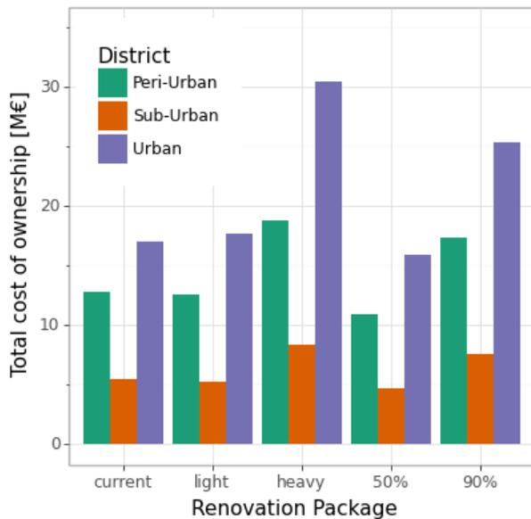
Figure 9 Total cost of ownership as function of the renovation packages, assuming a 30-year period and 3% discount rate
