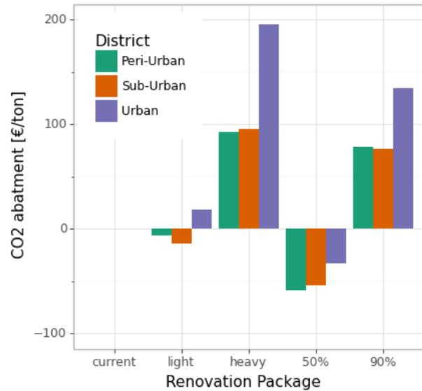
Figure 10 CO<sub>2</sub> abatement cost as function of the renovation packages. Only considering non-ETS emissions
