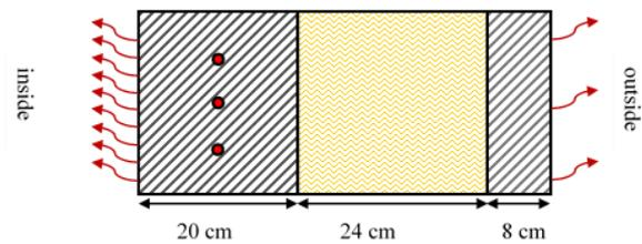
Figure 1: Layer composition of the TABS (cross section with solid load bearing layer with piping, insulation and outer layer from left to right).
