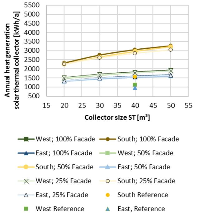
Figure 5: Heat generation: Solar thermal collector.
