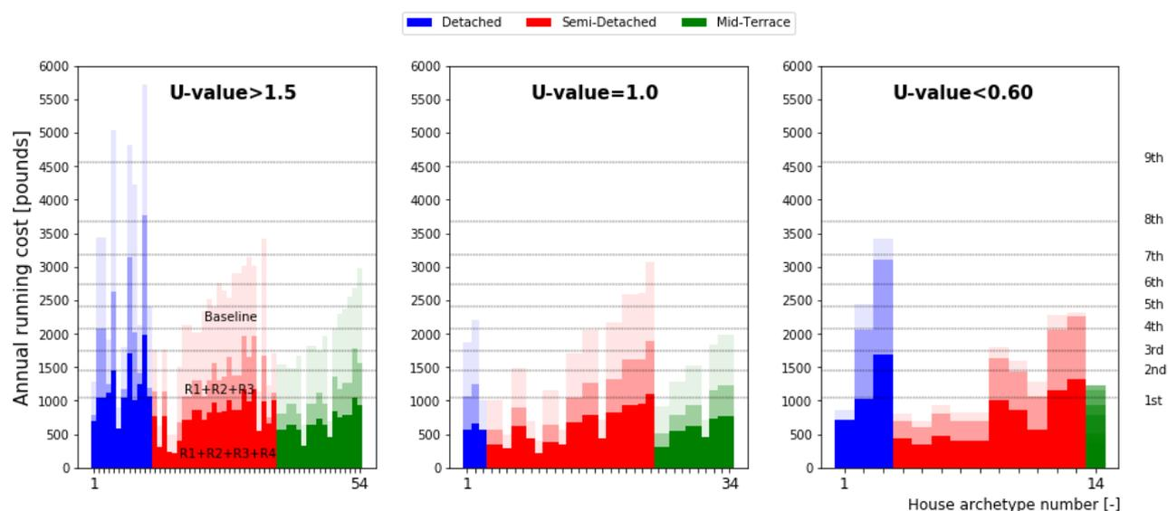
Figure 5: Annual running cost of the modelled house archetypes for baseline case, packaged fabric retrofit scenario (R1+R2+R3) and package fabric plus heating system retrofit scenario (R1+R2+R3+R4)
