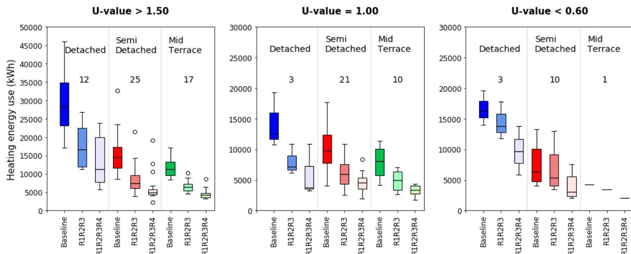
Figure 4: Distribution of the space-heating energy use per external wall insulation level and built form for baseline case and different retrofit scenarios
