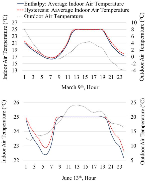
Figure 5 Hourly outdoor air temperatures and indoor air temperatures of the two methods on March 9<sup>th</sup> and June 13<sup>th</sup>
