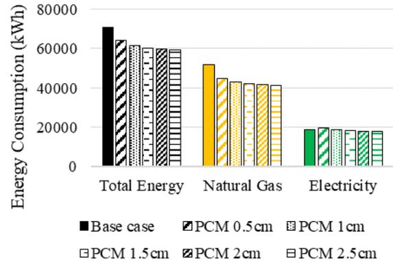
Figure 6 Energy consumptions of five PCM thicknesses
