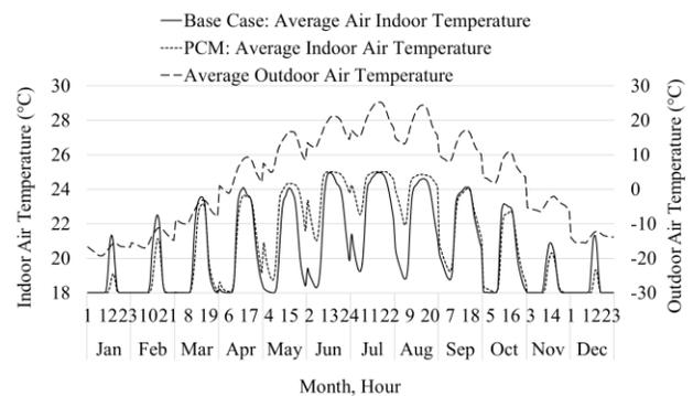
Figure 9 Hourly outdoor air temperatures and indoor air temperatures of the base and PCM cases
