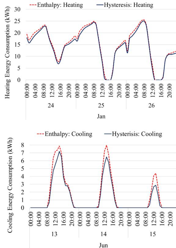
Figure 4 Hourly heating and cooling energy consumptions of the two methods from January 24<sup>th</sup> to 26<sup>th</sup> and from June 13<sup>th</sup> to 15<sup>th</sup>
