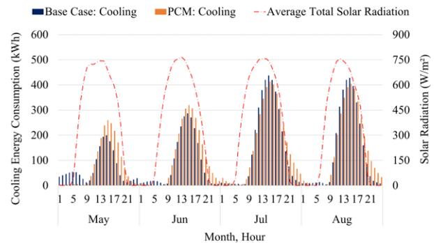
Figure 8 Hourly total solar radiation and cooling energy consumptions of the base and PCM cases
