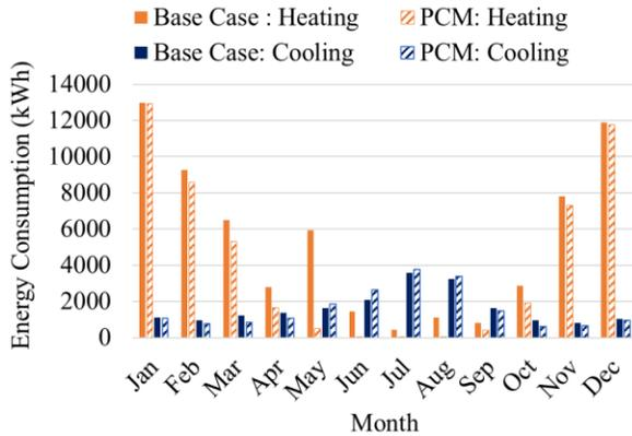
Figure 7 Monthly heating and cooling energy consumptions of base and PCM cases
