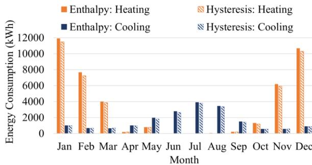
Figure 3 Monthly heating and cooling energy consumptions of the two methods
