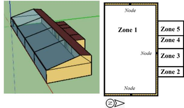
Figure 1 3D model and thermal zoning of the greenhouse
