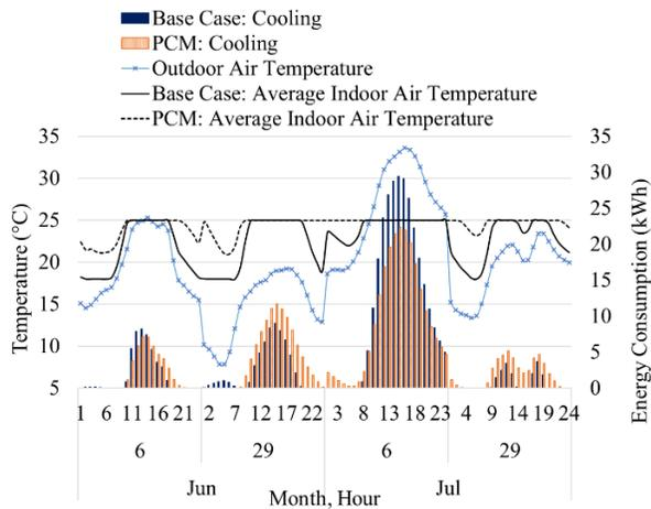
Figure 10 Hourly outdoor air temperatures, cooling energy consumptions, and indoor air temperature of the base and PCM cases
