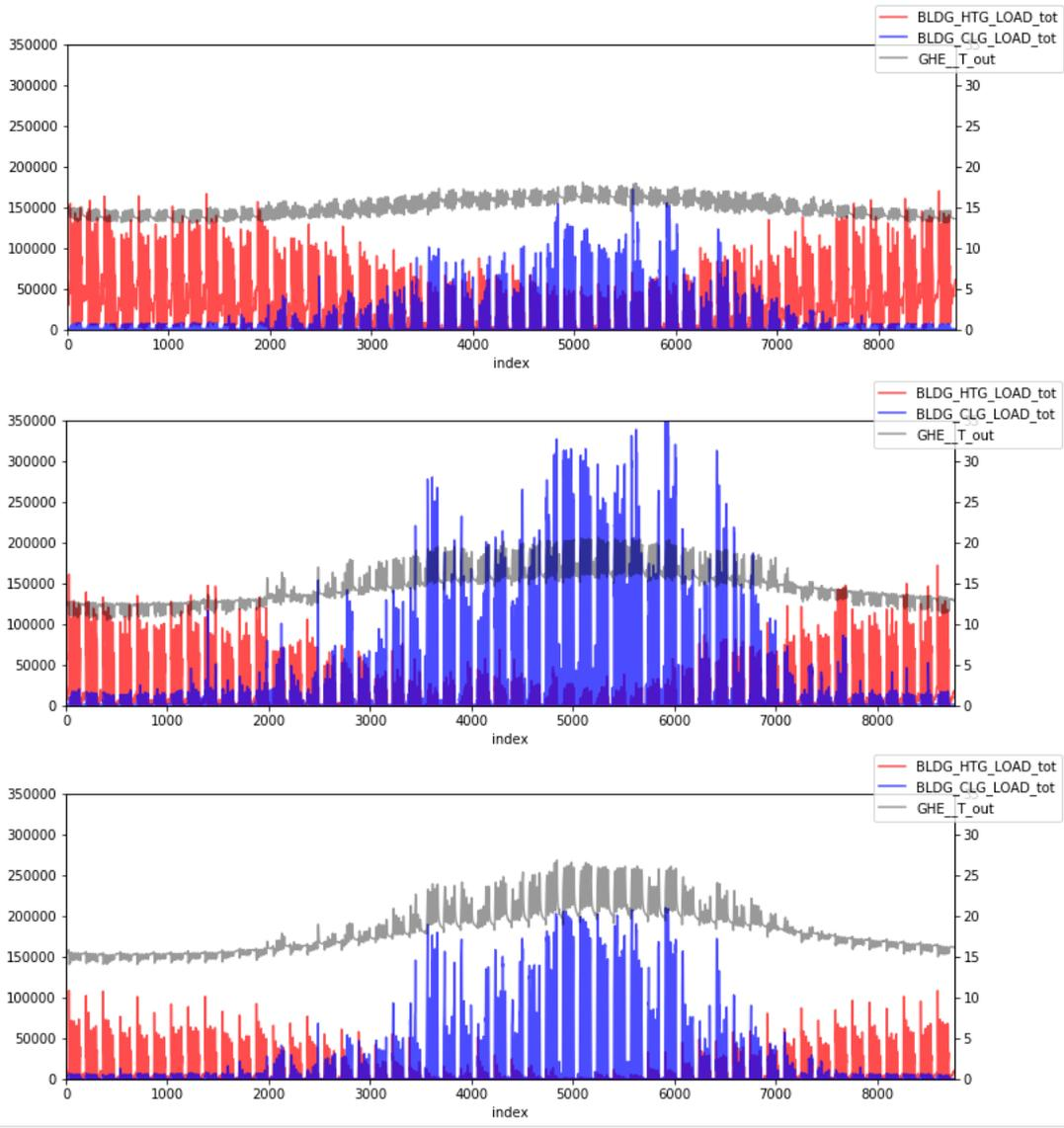
Figure 2: Annual heating and cooling load profiles with temperature of fluid leaving ground, (sample for 90<sup>th</sup>, 50<sup>th</sup>, and 10<sup>th</sup> percentile total heating demand)
