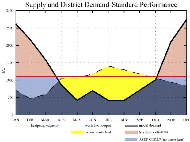
Figure 2: The model demand as it relates to the availability of waste heat and the capacity of the heat pumps.
