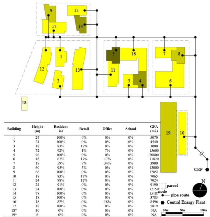
Figure 3: The 2D input for the CEA model includes footprints, heights, program. The node and pipe network can be manually added or created using a network analysis tool in the CEA.
