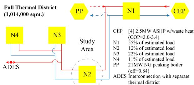
Figure 1: A diagram of the actual district heating system. The study is concerned with “N2” which is 12% of the estimated total load upon buildout.
