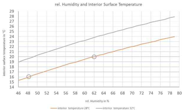
Figure 10. Maximum Relative Humidity and Interior Surface Temperature without Condensation
