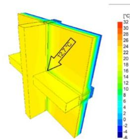
Figure 9 Coldest Point of the Window
