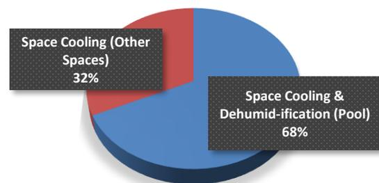
Figure 7. Cooling Load Breakdown.
