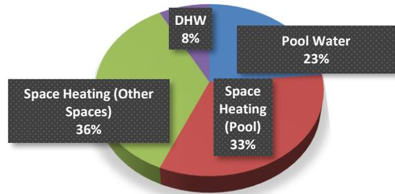
Figure 6. Heating Load Breakdown.
