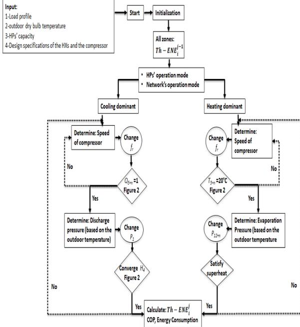
Figure 3 Logic flow chart to model CO<sub>2</sub> network
