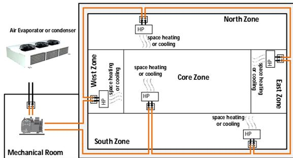
Figure 4: Hypothetical deployment of CO<sub>2</sub> network in a small office building with five thermal zones
