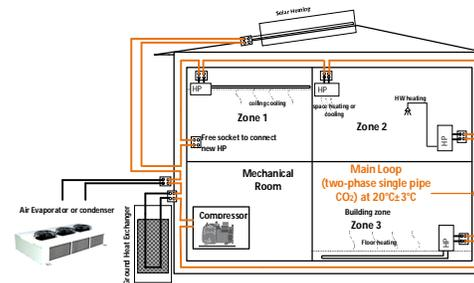
Figure 1 Schematic of a CO<sub>2</sub> Network in a building
