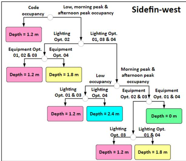
Figure 8: Sample decision tree demonstrates guidelines for selecting optimal sidefin shading size on west-facing façade.
