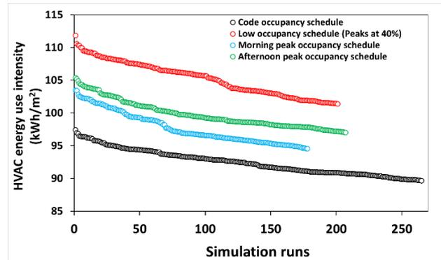
Figure 7: HVAC EUI of design optimization from four optimization runs using four different occupancy schedule scenarios. Each scatter plot represents an optimization run for an occupant scenario. The length of the scatter plot indicates where the optimization run converged to the optimal solution.
