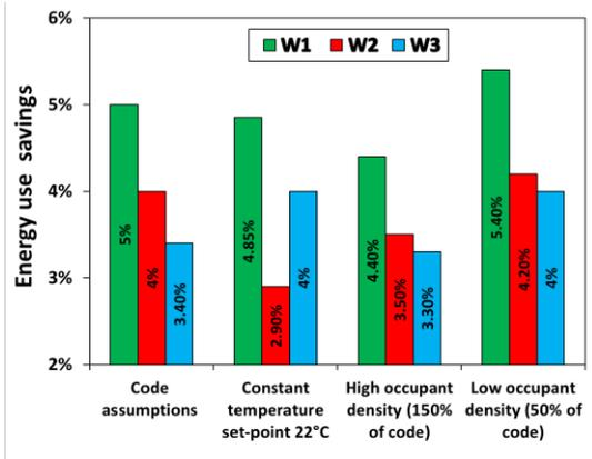
Figure 5: Sensitivity of energy saving potential from three window assemblies to the different occupant related assumptions. W1 ( $U=1.62 \text{ W/m}^2\text{K}$ ,  $SHGC=0.39$ ), W2 ( $U=2.04 \text{ W/m}^2\text{K}$ ,  $SHGC=0.58$ ), and W3 ( $U=1.47 \text{ W/m}^2\text{K}$ ,  $SHGC=0.25$ ).
