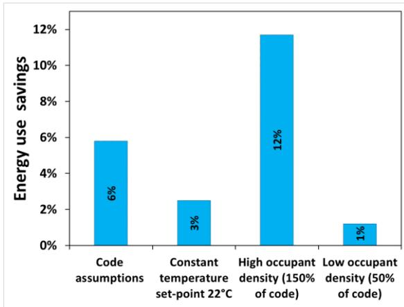
Figure 6: Sensitivity of energy saving potential from DCV to the different occupant related assumptions.
