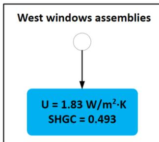
Figure 9: Sample decision tree demonstrates guidelines for selecting optimal window assembly material for west-facing façade.
