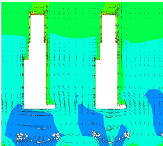
**Fig. 5. PPD index for swirl inlet diffuser**
