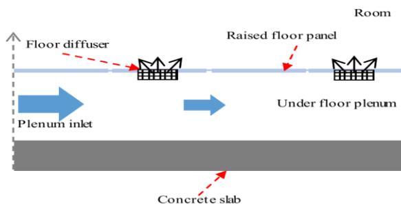
Fig. 1. Under floor plenum schematic
