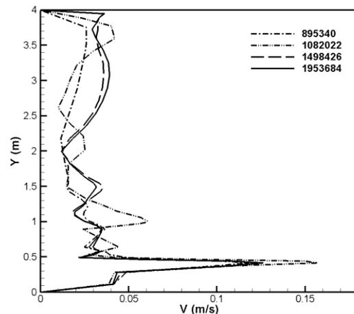
**Fig. 3. Grid independency check for velocity along; x=4.0 and z=-1.3**
