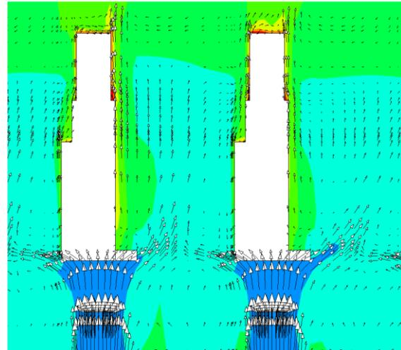
**Fig. 6. PPD index for direct inlet diffuser**
