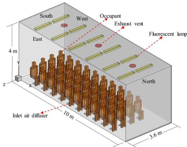
**Fig. 2. Configuration of the model space with a symmetry wall**
