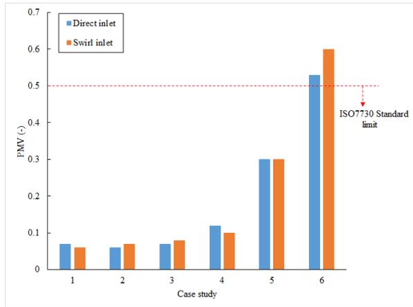
**Fig. 4. PMV index for both of the inlet diffusers**
