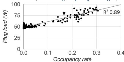
Figure 8: The relationship between occupancy and mean plug load per occupant (built using output of `occ2plug`). The `LightWrtSolRad` function builds a Bernoulli lighting model with the predictor solar radiation on the façade. It predicts the probability of finding the
