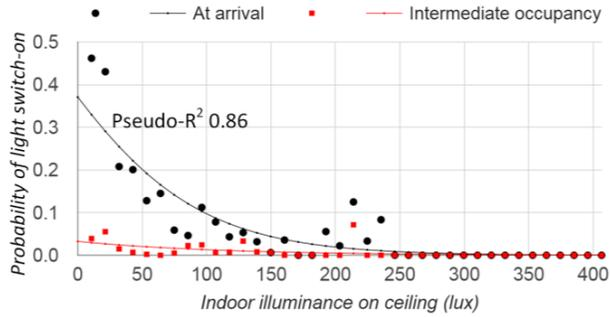
Figure 14: Discrete-event Markov light switch-on models (built from *LightSwitchWrtIndLuxArr* and *LightSwitchWrtIndLuxInt*). The scatter points represent likelihood weights and straight lines are the logistic regression fit.
