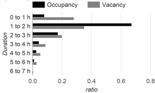
Figure 6: Survival models predicting the duration of occupancy and vacancy periods (built using outputs of `occ2durpre` and `occ2durabs` functions).
