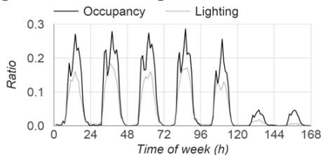
Figure 2: Mean weekly occupancy and lighting schedules (built using outputs of occ2sch and light2sch functions).
