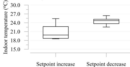
Figure 16: The indoor temperature distribution at the thermostat setpoint increase and decrease instances (built using output of *TstatUseWrtlat*).
