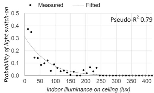
Figure 13: Discrete-time Markov light switch-on model using indoor illuminance as the predictor (built using output of `LightSwitchWrtIndLux`) (timestep size 15 min).
