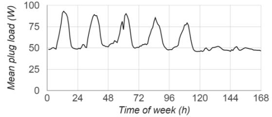
Figure 3: Mean weekly plug load schedule per occupant (built using output of plug2sch function).
