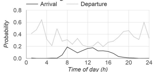
Figure 5: Discrete-time Markov occupancy model predicting the likelihood of arrival (if the space is unoccupied) and departure (if the space is occupied) in the next one hour (built using MarkovArrDpt function).
