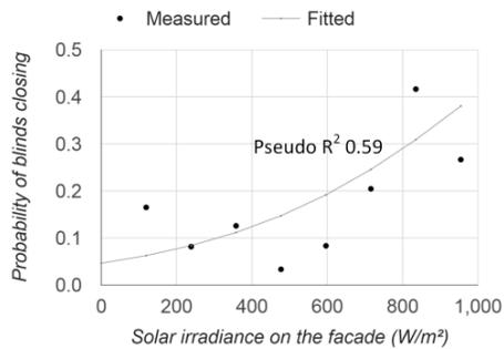
Figure 12: Discrete-time Markov blinds closing model using solar irradiance as the predictor (built using output of `BlindClosingWrtSolRad`) (timestep size 30 min).
