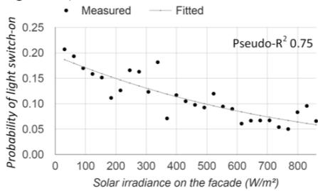
Figure 11: Discrete-time Markov light switch-on model using solar irradiance as the predictor (built using output of `LightSwitchWrtSolRad`) (timestep size 15 min).
