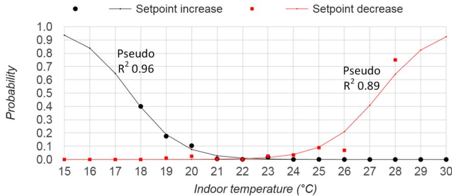
Figure 17: Discrete-time Markov thermostat use models (built using output of MarkovTstat). The scatter points represent discrete likelihood weights and the straight lines are the logistic regression fit.
