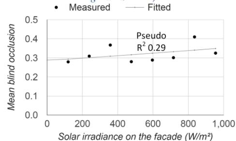
Figure 10: Bernoulli blind occlusion model (built using output of `BlindWrtSolRad`).
