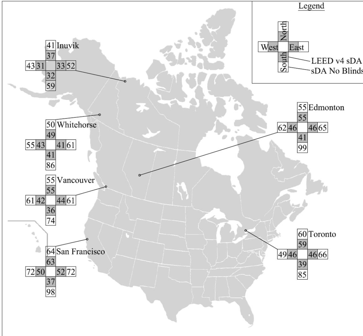
**Figure 2** –Simulation results for % of floor area achieving sDA targets with and without glare control devices/ blinds
