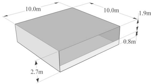
**Figure 1** – Geometry of modelled office space. For daylight simulation results in each cardinal direction, this geometry is rotated so that the window is facing the respective direction
