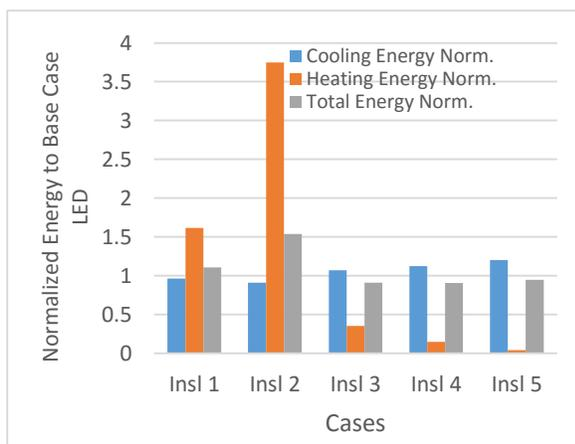
**Figure 5:** Effect on Energy Consumption by Modifying the Insulation Values from Code. Insl 1: 80%; Insl 2: 50%; Insl 3: 150%; Insl 4: 200%; Insl 5: 300%
