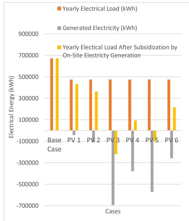
**Figure 10:** Effect on Energy Consumption by the Utilization of Photovoltaics. Refer to section 3.7 for implementation scenarios of the BIPV systems being investigated.
