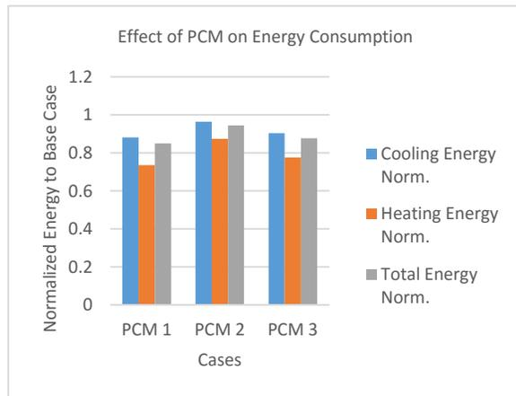
**Figure 8:** Effect of Energy Consumption by use of Phase Change Material. Comparing EnergyPlus Database Supplied PCM (PCM 1) to Macro-Encapsulated Dodeconal PCM (PCM 2) and Micro-Encapsulated DuPont Energain PCM (PCM 3)
