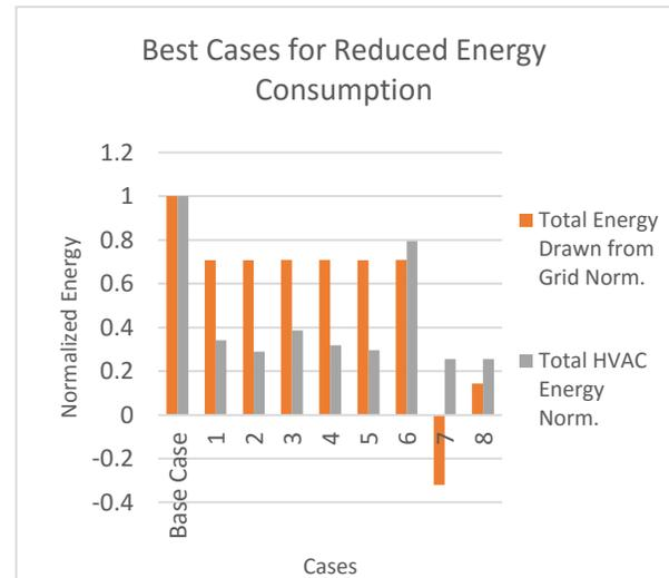
**Figure 11:** Energy Performance of Best Case Models. See Table 4 for case descriptions. Case 54 has 150% of required energy generated on site. Base Case model shown here for comparison is one with fluorescent lighting.
