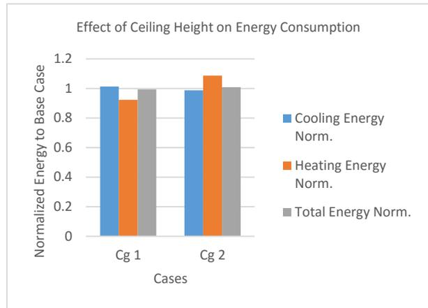
**Figure 6:** Effect on Energy Consumption by Changing the Ceiling Height. Base Case has ceiling height of 4.27 m; Cg 1 has ceiling height of 5.27 m; Cg 2 has ceiling height of 3.27 m
