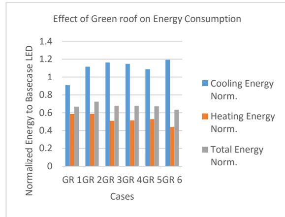
**Figure 9:** Effect on Energy Consumption with Different Green Roof Compositions. Refer to section 3.6 for green roof compositions being investigated.
