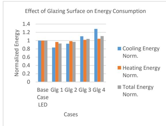
**Figure 7:** Effect on Energy Consumption by Changing the Size of Glazing Surface on South Facade. All cases use LED lighting. 20%, 0%, 10%, 30% and 50% glazing surfaces in cases, respectively.
