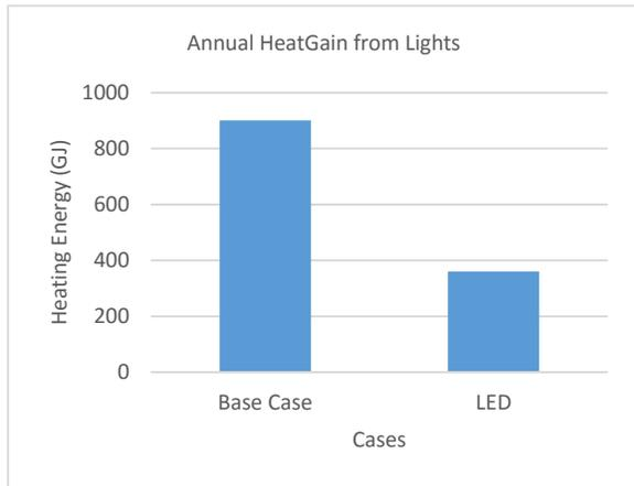
**Figure 4:** Heat Gain from Lighting Annually. Base case uses fluorescent tubing lights which are associated with higher levels of radiant heat.
