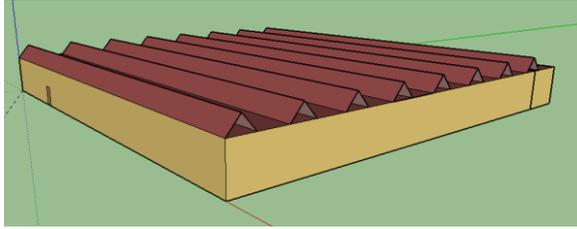
**Figure 2:** Supermarket design with Saw-Tooth structures for increased solar performance (SketchUp Model)
