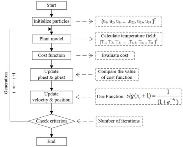
Fig.4 Flow chart of DPSO-MPC
