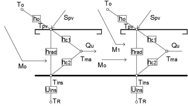
Figure 4: Multiple-inlet BIPV/T energy balance.
