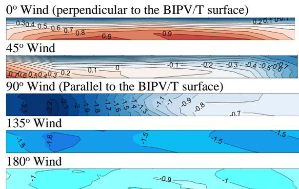
Figure 8: Pressure coefficient distributions on BIPV/T area. From top to bottom: 0°, 45°, 90°, 135° and 180° angles of incidence of wind.
