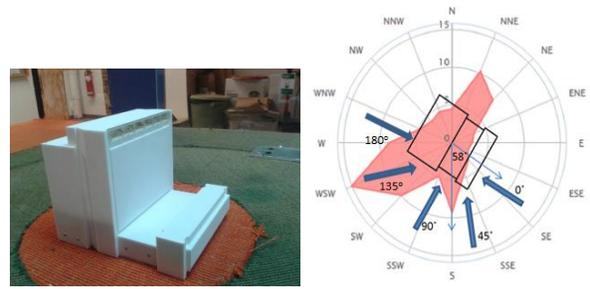
Figure 6: 1:400 scaled model of the building (left) and building orientation, wind diagram for Montreal and wind directions tested (right).
