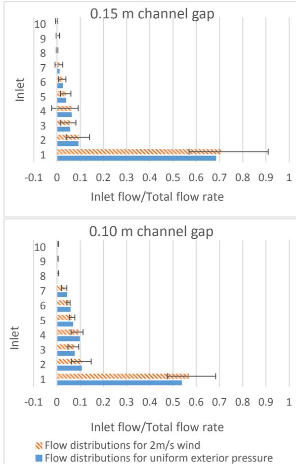
Figure 9: Normalized flow distributions of multiple-inlet systems with a 0.15 m and 0.10 m channel gap, for 2 m/s wind at 45° angle of incidence and 400 kg/h total flow rate.
