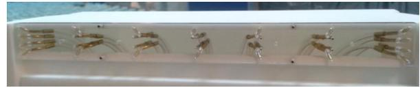
Figure 7: BIPV/T façade for the wind tunnel model, equipped with pressure taps.
