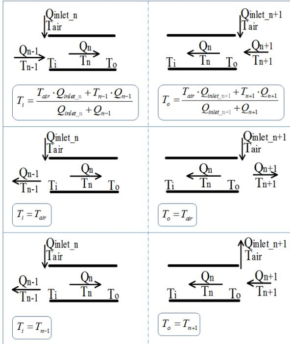
Figure 5: The six possible channel flows and channel air temperature inlet boundary conditions.
