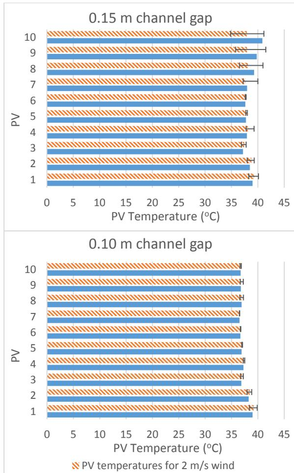
Figure 10: PV temperature distributions of multiple-inlet systems with a 0.15 m and 0.10 m channel gap, for 2 m/s wind at 45° angle of incidence and 400 kg/h total mass flow rate.
