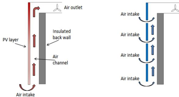
Figure 1: Single and multiple-inlet BIPV/T system.
