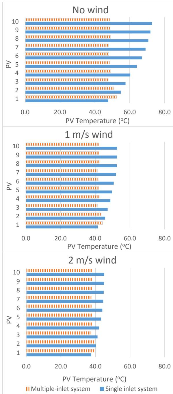
Figure 11: Comparison of PV temperatures for single and multiple-inlet systems for no wind, 1 m/s and 2 m/s wind and 400 kg/h total mass flow rate.
