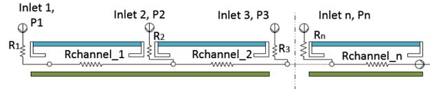
Figure 2: Electrical resistance analogy for flow modelling of a BIPV/T system with multiple openings.
