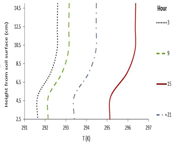
Figure 3- Plant temperature profile in 6-hour period in 24 hours
