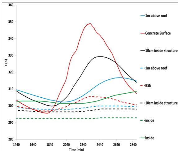
**Figure 4- Comparison of temperatures of green roof and conventional roof**
