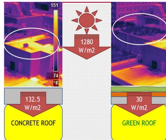
**Figure 5- Comparison of heat flux transmission in green roof and concrete roof**
