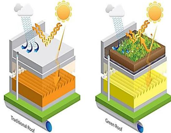
**Figure 1- heat dissipation in green roof in contrast with conventional roof**
