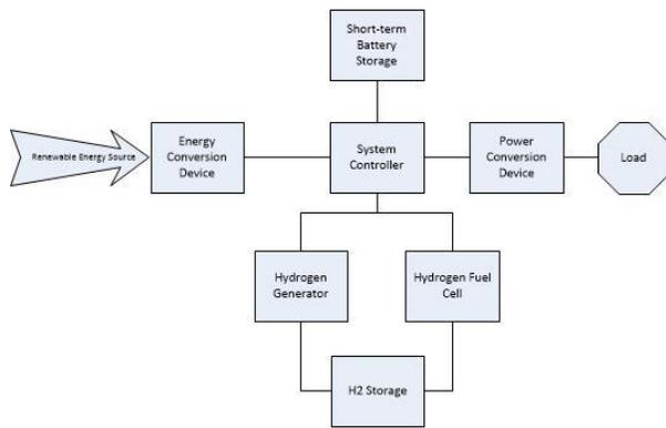
Figure 1: General architecture of a solar-hydrogen energy system.
