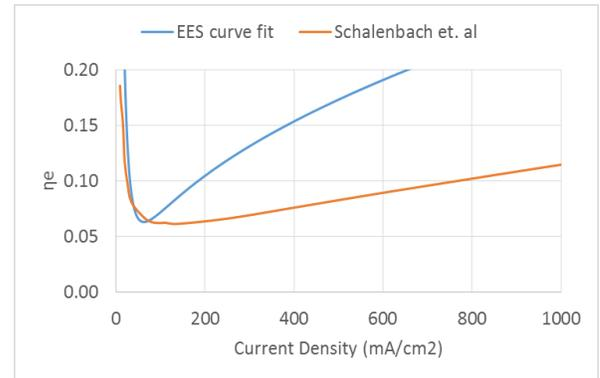
Figure 5: Comparison of Schalenbach's data and EES curve fit. The drastic divergence past 100mA/cm2 is due to differences in ohmic resistances of the cells, unrelated to the Faraday efficiency.
