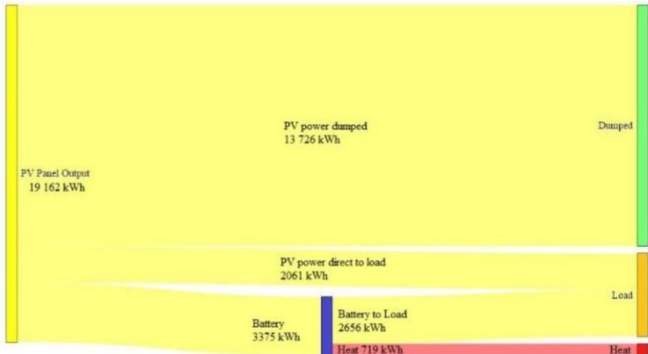
Figure 9: Sankey diagram of energy flows in the all-battery system. Note the large portion of solar energy that goes unused.
