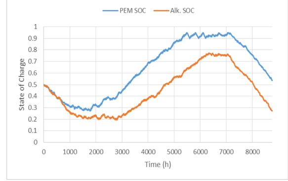
Figure 6: State of charge (SOC) of the hydrogen storage tank for 2 simulated systems; PEM electrolyzer (blue), and alkaline electrolyzer (orange)
