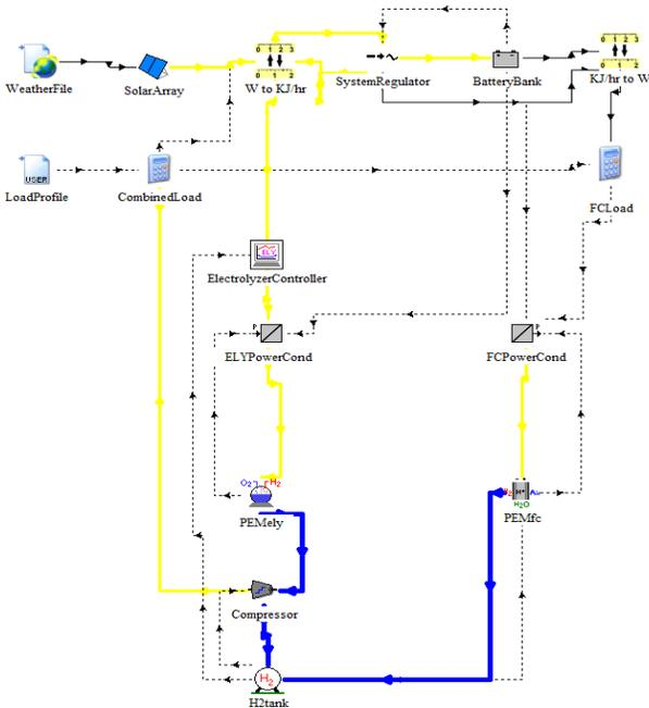
Figure 2: Graphic representation of the simulated system in TRNSYS (i.e., Screen-capture). Yellow represents flows of electric power, blue shows flows of hydrogen gas, and dashed lines are signals.
