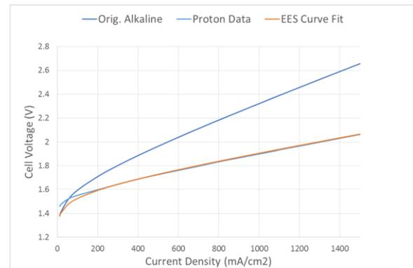
Figure 4: Comparison of manufacturer's data and EES curve fit results.
