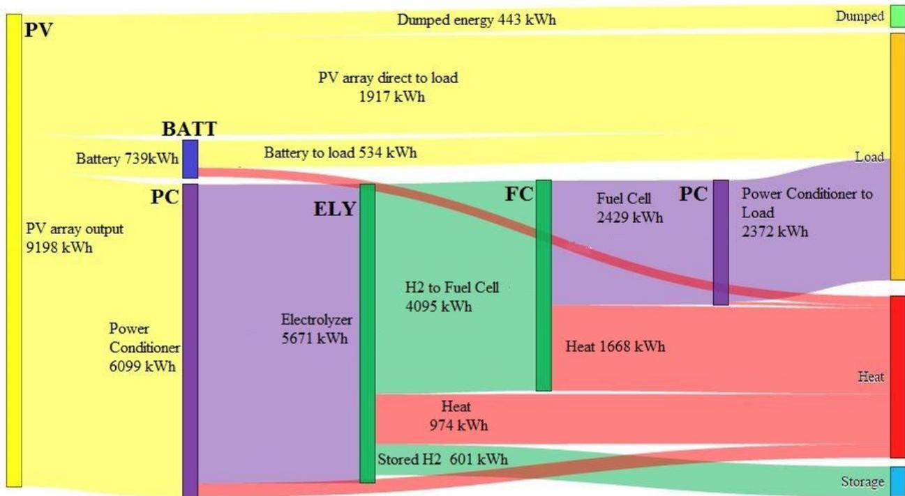
Figure 7: Energy flows through the solar-hydrogen energy storage system
