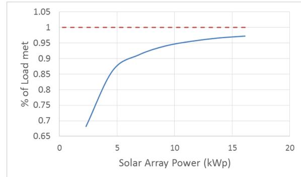
Figure 8: sensitivity analysis of solar array size for all-battery system
