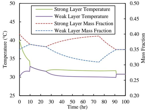
**Fig. 4.** TYPE 301 operation when forced to mix, re-stratify and then mix again.
