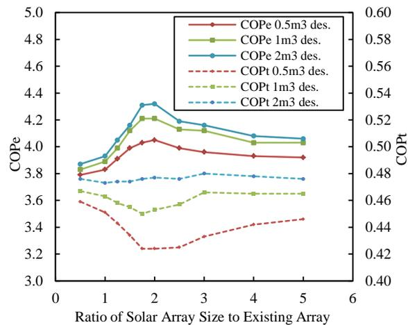
**Fig. 6.** COPs of systems simulated using different sized solar arrays and desiccant storage tanks.
