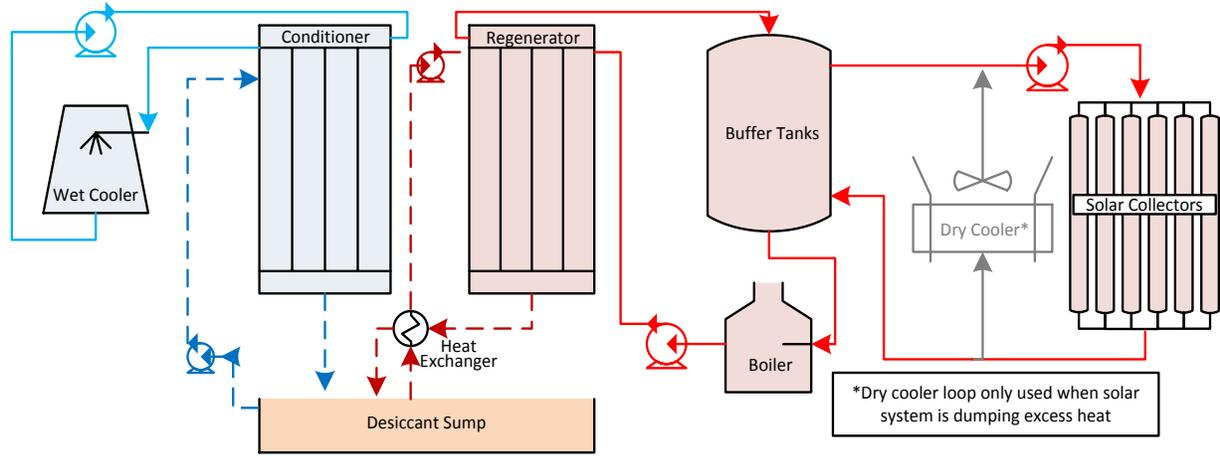
Fig. 1. Simplified system layout showing the LDAC unit and the associated heat generation and rejection sub-systems.
