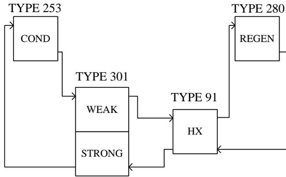
**Fig. 2.** A simplified schematic of the desiccant storage tank showing the weak and strong layer, and its connections to the LDAC components.
