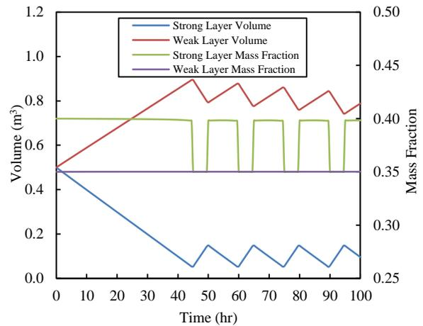
**Fig. 3.** TYPE 301 operation when forced to empty the strong layer. Layer is shown to be re-established before being emptied again repeatedly.
