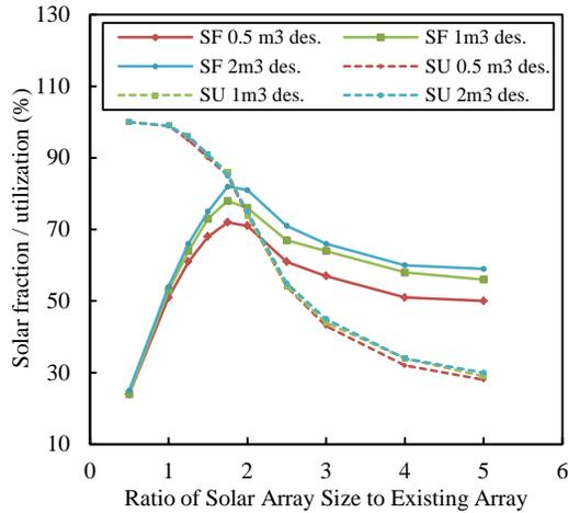
**Fig. 5.** Solar fraction and solar utilization ratios of systems simulated using different sized solar arrays and tanks.
