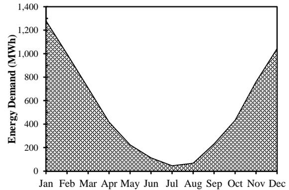
Figure 4: Annual heat load characteristics of the proposed DE system
