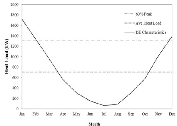
*Figure 1: Comparison of two sizing methods for the DE system. Data are for a typical DE system operating in the Canadian climate*
