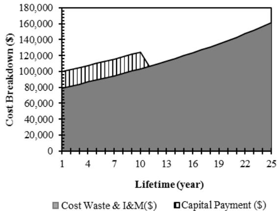
Figure 14: WTE plant cost breakdown
