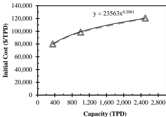
Figure 11: Cost curve for WTE plants with plant capacity, and curve fitting equation
