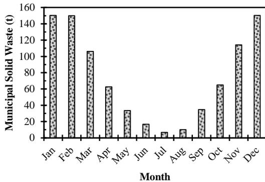
Figure 10: Monthly waste needed by WTE plant to satisfy DE system heat demand
