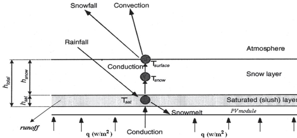
Figure 1: Heat transfer in the three-node snowmelt model
