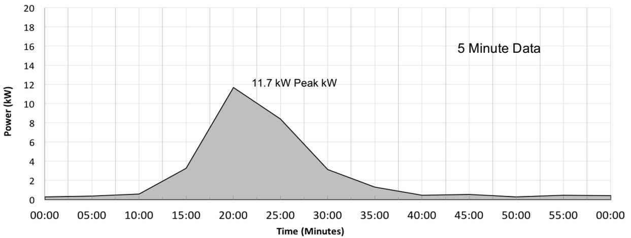
Figure 9. 60 minutes of electricity load data from a residential dwelling, representing supper-hour on-peak activity measured March 10, 2016, showing 1 s, 1 min, and 5 min data capture.
