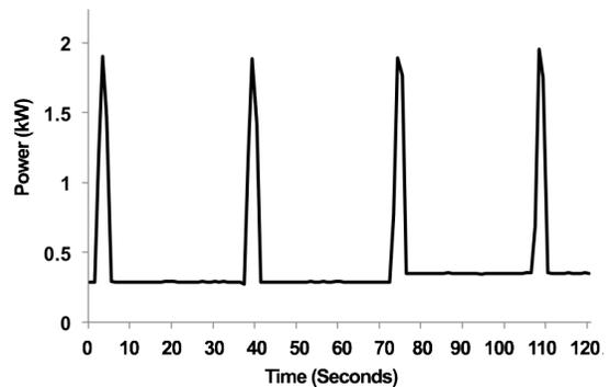
**Figure 5. Pulse-modulated electricity demand**
