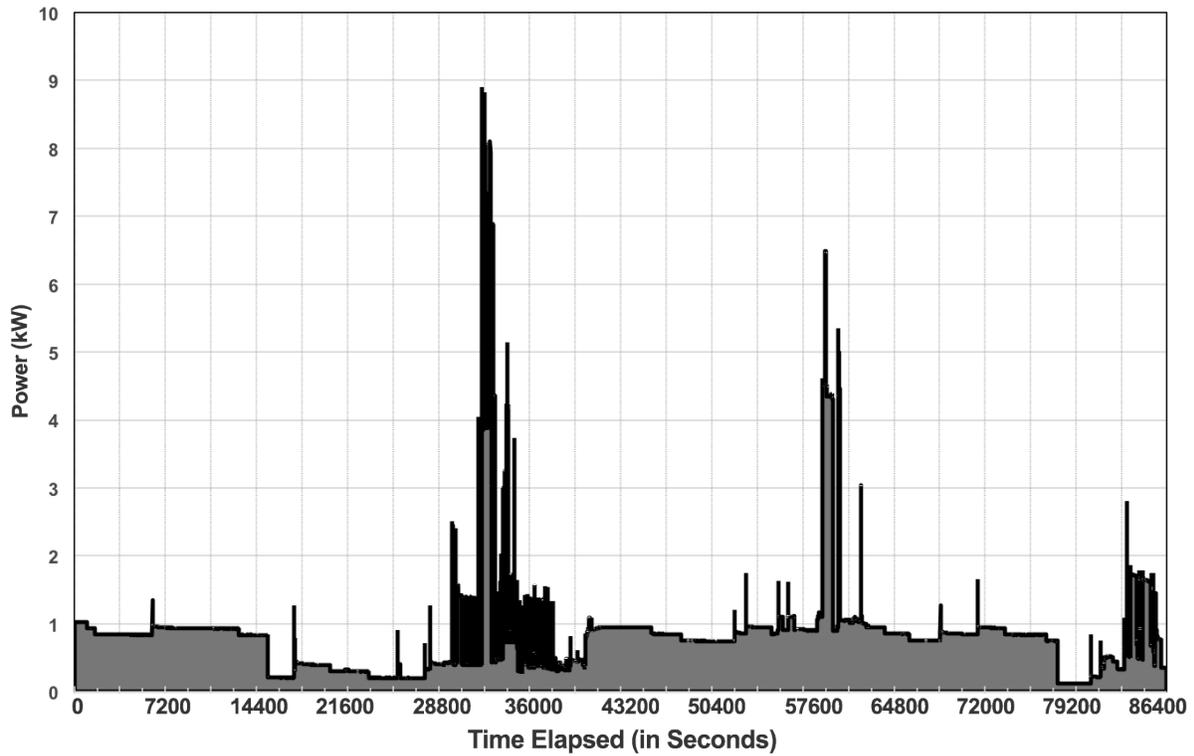
Figure 7. 24-hours of 1-second electricity load data from a residential dwelling, measured August 1, 2015.
