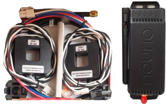
**Figure 2. Current transducers (CTs), and a Wi-Fi microprocessor-based electricity monitor.**
