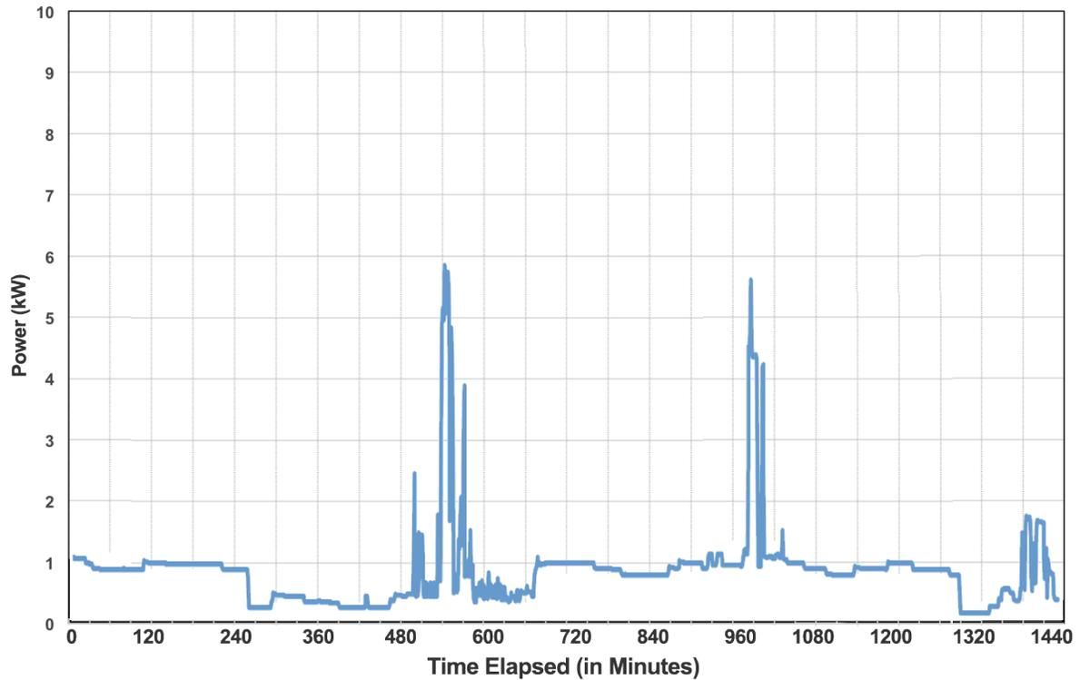
Figure 8. 24-hours of 1-minute electricity load data from a residential dwelling, measured August 1, 2015.
