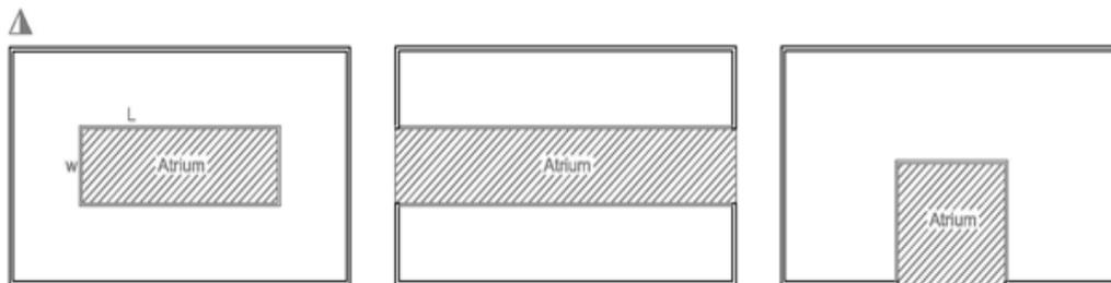
Figure 2 Atrium types plan view (left to right): central, attached and semi-enclosed (Huang, 2003)
