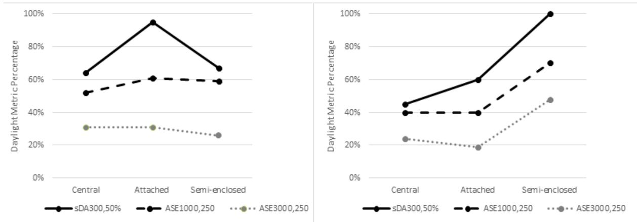
Figure 5 Comparison of average dynamic daylight metrics among atrium types with WI=0.5 (left) and WI = 1 (right) using skylight roof (climate zone 3)
