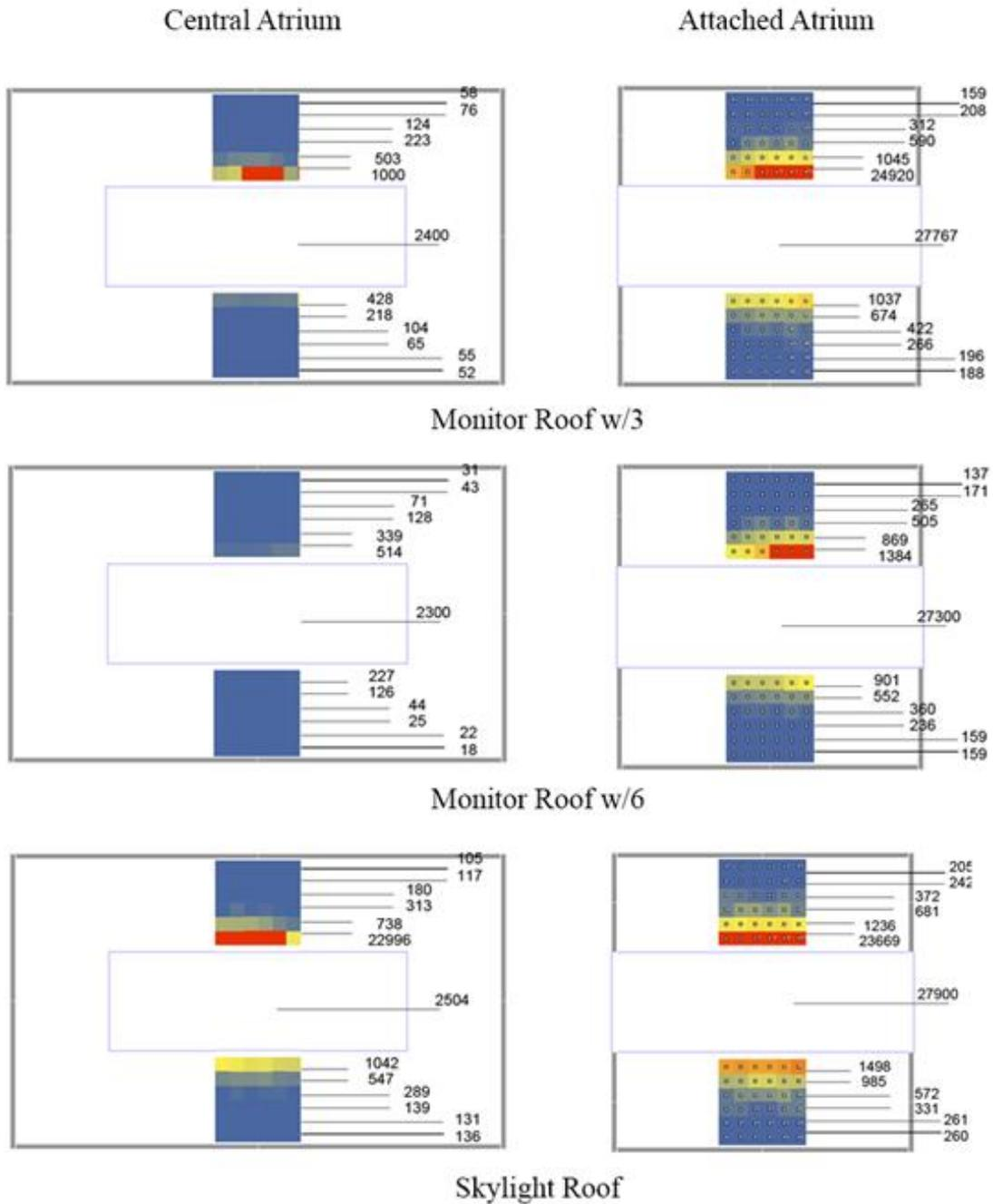
Figure 4 Point-in-time analysis of atrium buildings for WI=1 on Dec 21st at 9:00 a.m. under clear sky with sun
