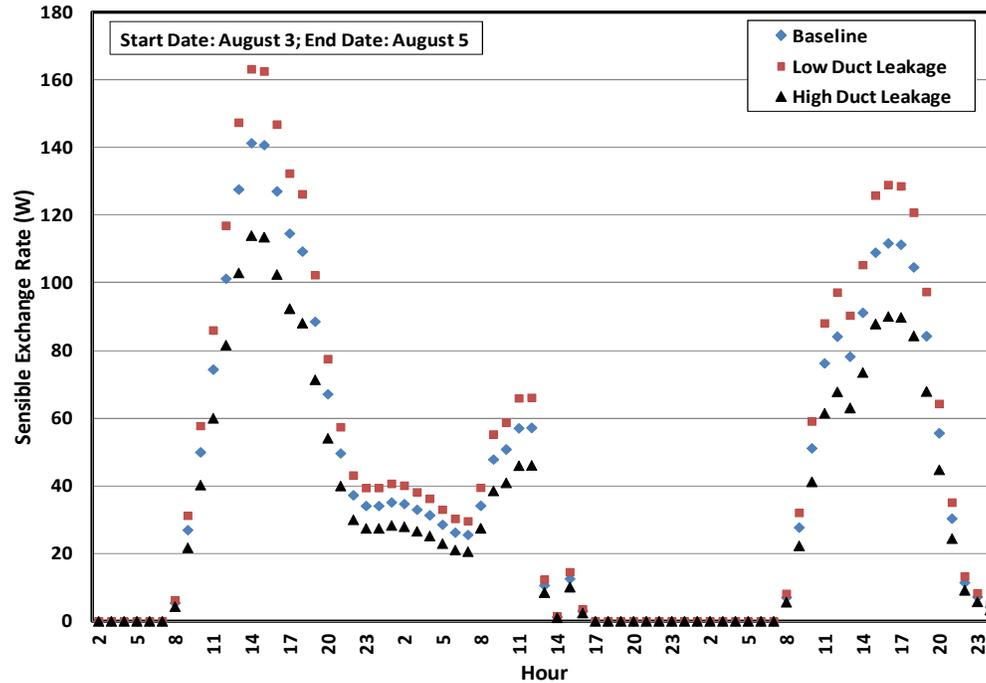
Figure 4 – Summer recovered sensible cooling as a function of leakage flow.
