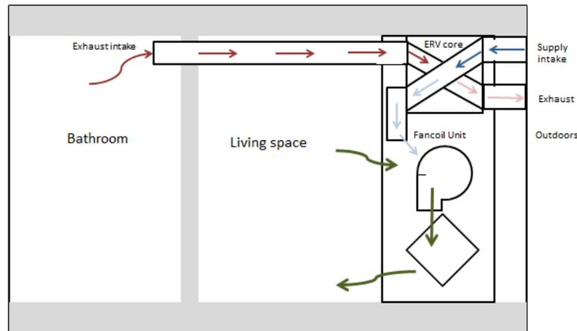
**Figure 1 - In suite mechanical system layout**
