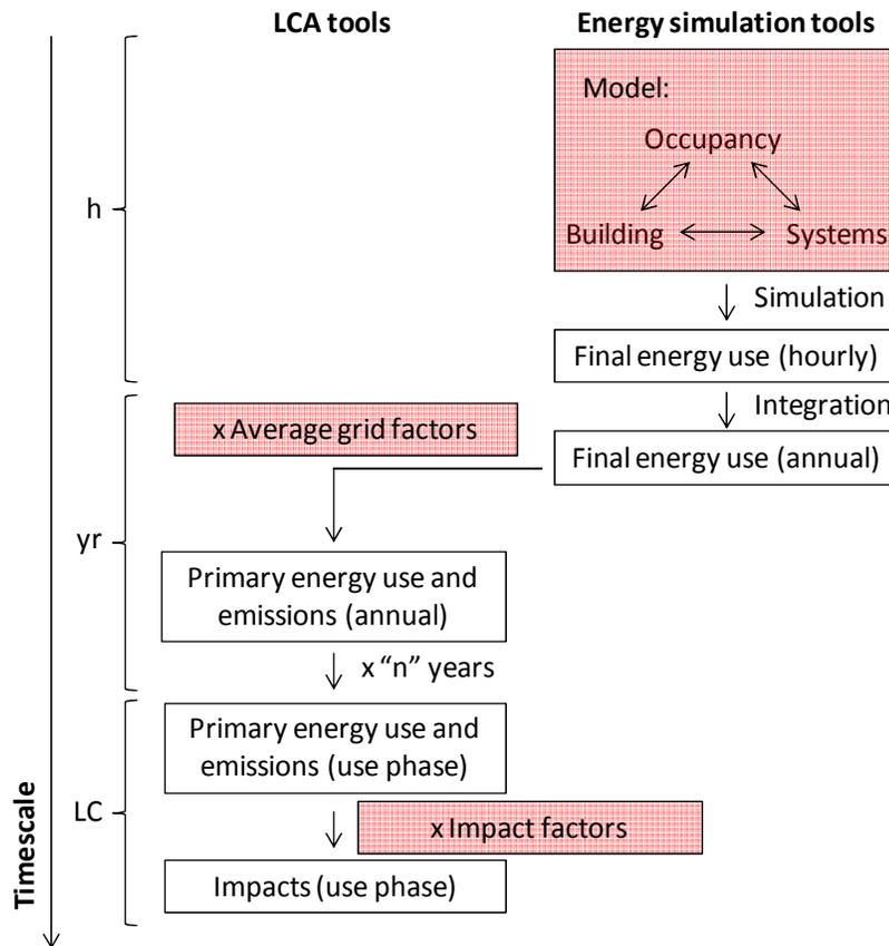
**Figure 2 – Typical use of tools for use phase impact evaluation. Shaded boxes show steps that require input data**
