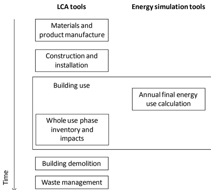
**Figure 1 – Typical use of tools in different stages of a whole building LCA**
