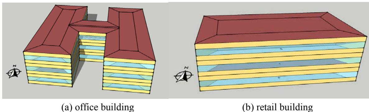
**Figure 2: The 3-D EnergyPlus models for an office building and a retail building**
