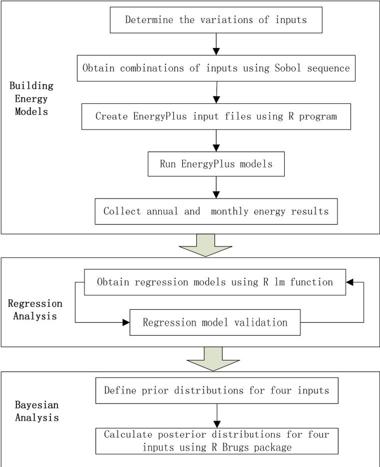
**Figure 1: The flow chart for input parameter estimation using regression models and Bayesian analysis**
