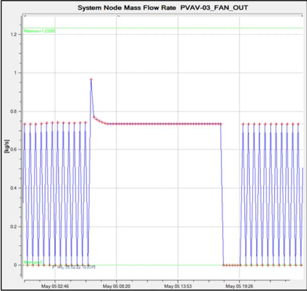
**Figure 8: Fan Operation Sample Day Check**
