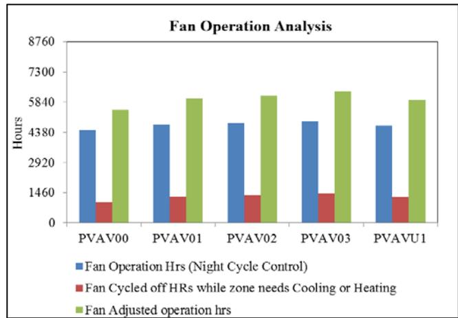
**Figure 5: Fan Operation Analysis**
