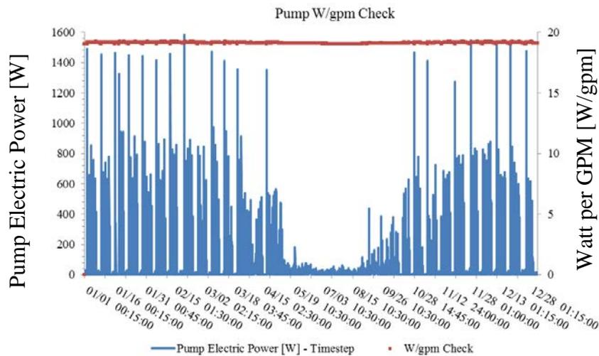
**Figure 2: Baseline Pump 19 W/gpm Check**
