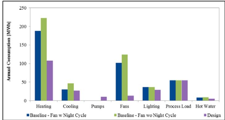
**Figure 9: Energy Usage Comparison for Different Fan Operation Controls**
