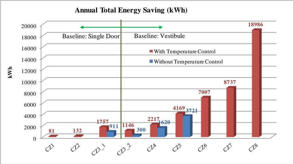
**Figure 4: The national annual total saving of air curtain in kWh when compared to the single door and/or the vestibule**
