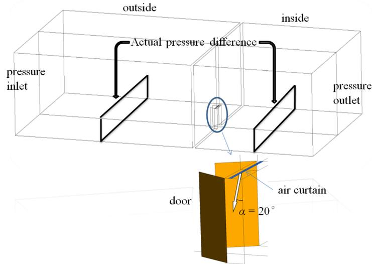
**Figure 2: CFD model of the building section with the air curtain**
