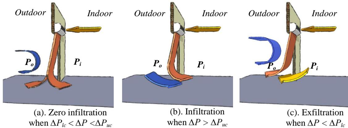
**Figure 1: Infiltration/exfiltration characteristics of an air curtain jet under different pressure differences,  $\Delta P = P_o - P_i$  (note that the zero infiltration does not apply to the air recirculating through the air curtain)**
