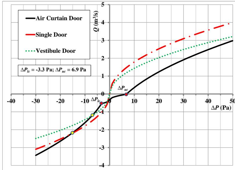
**Figure 3: Infiltration/Exfiltration characteristics of air curtain door when the air curtain is in operation when compared to single door and vestibule door (Yuill, 1996)**
