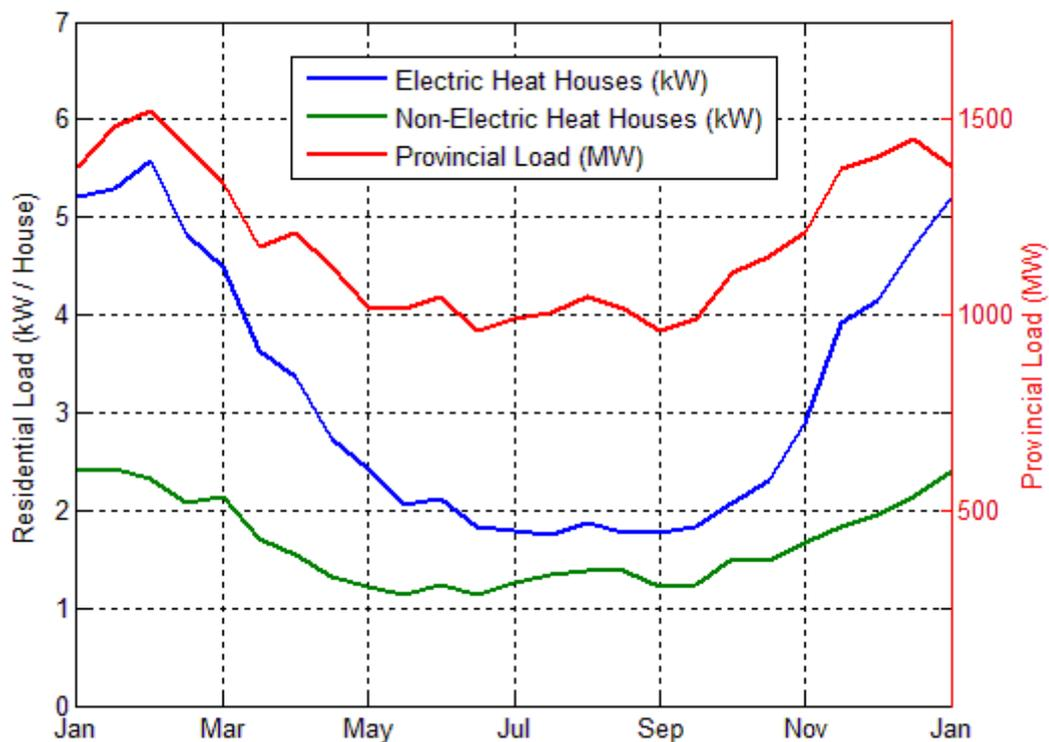
**Figure 2: Monthly average electricity demand of the three house types in comparison with total provincial load**
