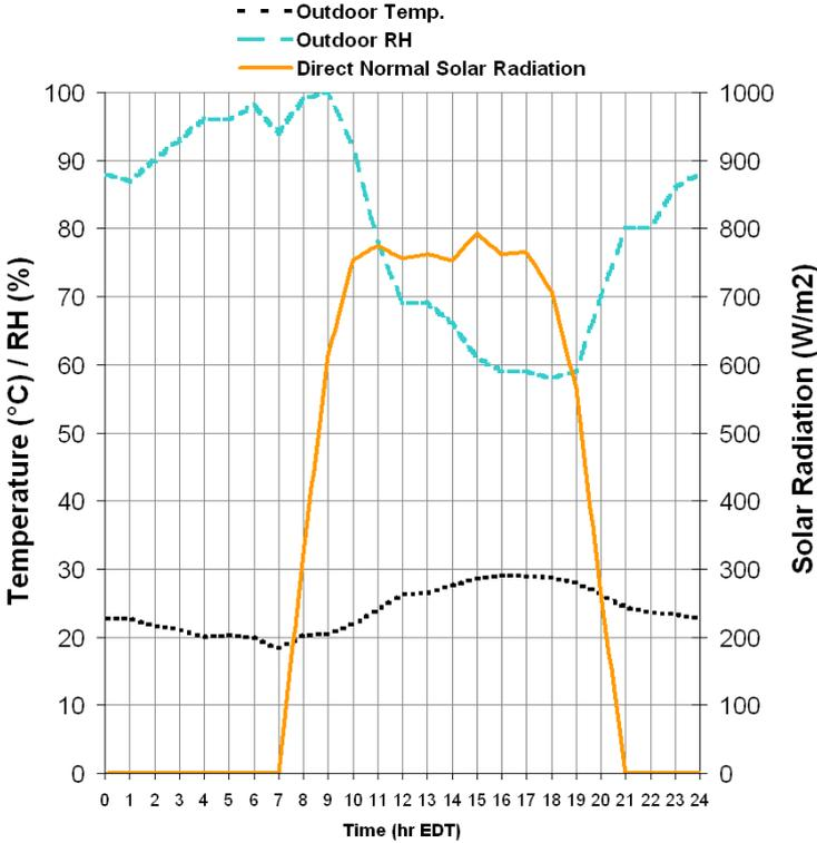
Figure 2: Weather data used in the ESP-r model. Data is from August 31<sup>st</sup>, 2000, Toronto.
