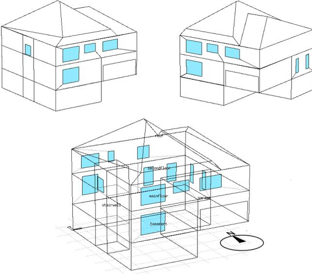
Figure 1: Geometry of CCHT house model in ESP-r (windows shaded blue).
