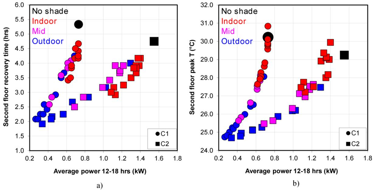
**Figure 7: Averaged power between 12:00-18:00 hours vs. a) second floor recovery time and b) second floor peak temperature for zoned control scenarios C1 and C2 (shade layer position indicated by marker colour).**
