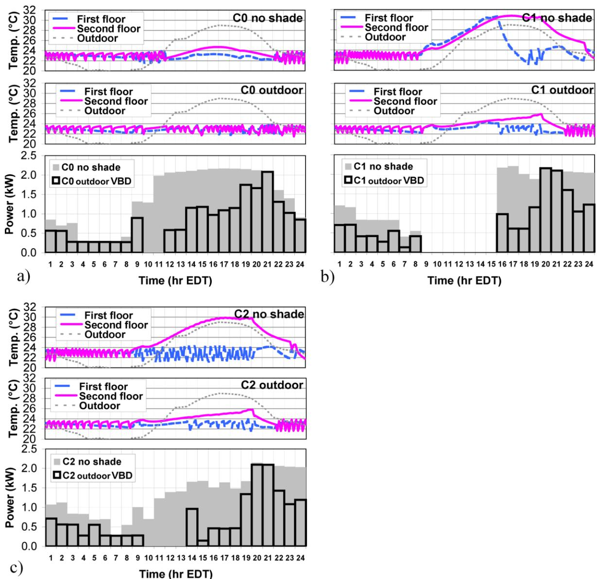
Figure 4: Temperatures and hourly averaged cooling power for unshaded vs. outdoor Venetian blind cases subject to the three zoned control scenarios a) C0, b) C1 and c) C2.
