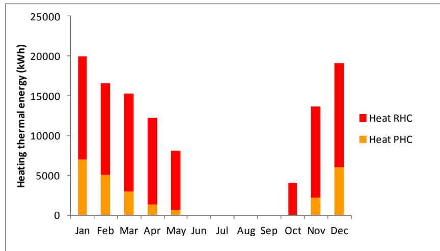
**Figure 11 – Control logic 2 results. Heating thermal energy use. PHC is energy use in the preheating coil (1<sup>st</sup> stage of conditioning), RHC is energy use in the reheating coil (2<sup>nd</sup> stage of conditioning)**
