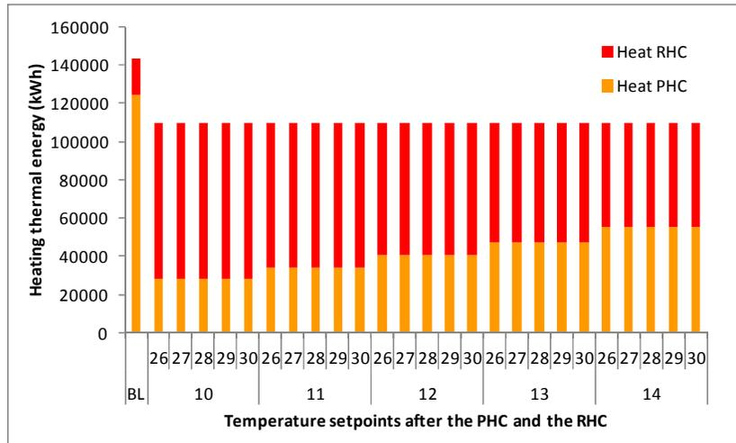
**Figure 7 – Control logic 1 results. Heating thermal energy use. PHC is energy use in the preheating coil (1<sup>st</sup> stage of conditioning), RHC is energy use in the reheating coil (2<sup>nd</sup> stage of conditioning)**
