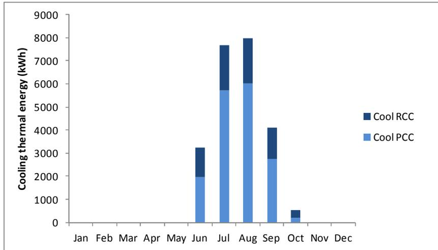
**Figure 12 – Control logic 2 results. Cooling thermal energy use. PCC is energy use in the precooling coil (1<sup>st</sup> stage of conditioning), RCC is energy use in the recooling coil (2<sup>nd</sup> stage of conditioning)**
