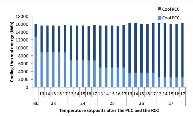
**Figure 9 – Control logic 1 results. Cooling thermal energy use. PCC is energy use in the precooling coil (1<sup>st</sup> stage of conditioning), RCC is energy use in the recooling coil (2<sup>nd</sup> stage of conditioning)**
