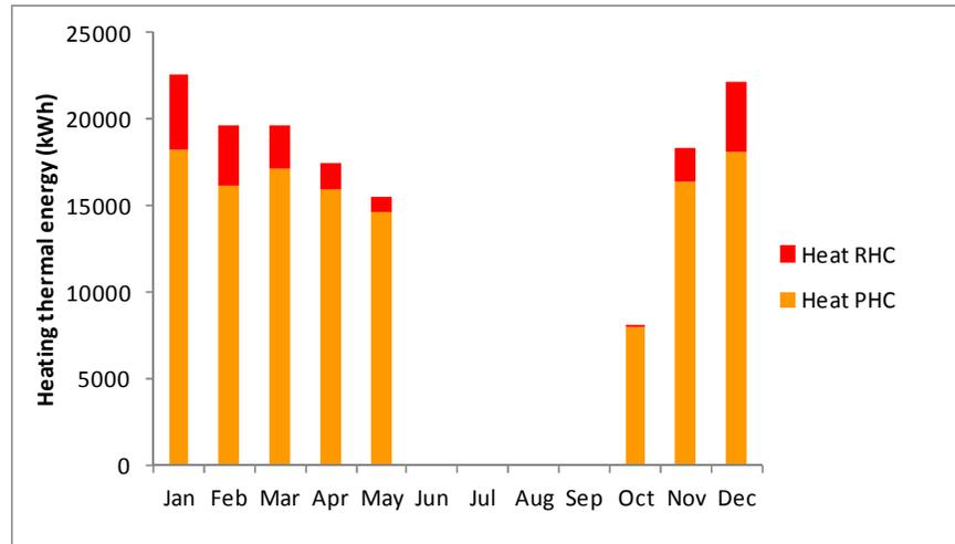
**Figure 3 – Baseline results. Heating thermal energy use. PHC is energy use in the pre-heating coil (1<sup>st</sup> stage of conditioning), RHC is energy use in the reheating coil (2<sup>nd</sup> stage of conditioning)**
