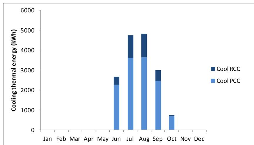
**Figure 4 – Baseline results. Cooling thermal energy use. PCC is energy use in the pre-cooling coil (1<sup>st</sup> stage of conditioning), RCC is energy use in the recooling coil (2<sup>nd</sup> stage of conditioning)**
