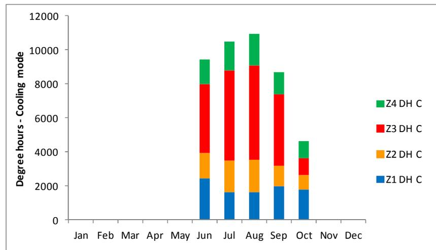
**Figure 6 – Baseline results. Degree hours in cooling mode**
