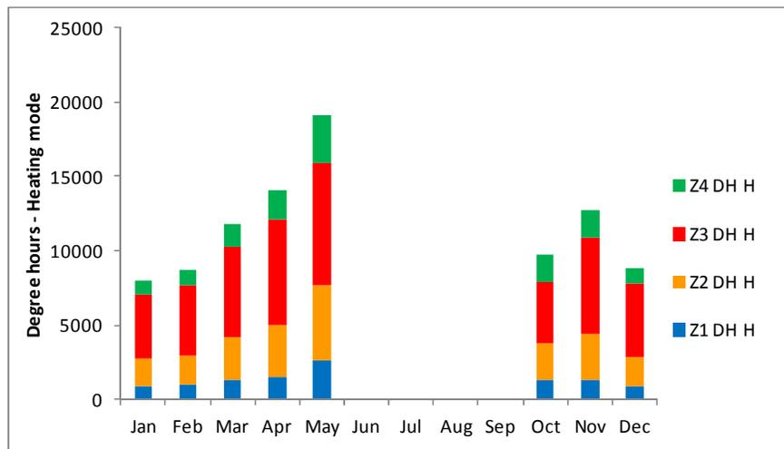
**Figure 5 – Baseline results. Degree hours in heating mode**
