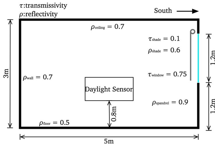
**Figure 3: Elevation view of office space modelled in EnergyPlus**
