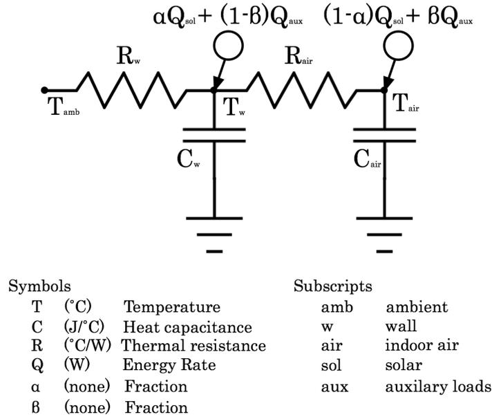
**Figure 2: RC model representation of building model**
