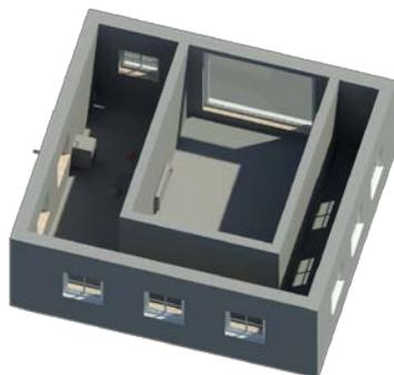
Figure 3: Use Case Room, based on VDI 6007 with simple Heating-System as shown in figure 2
