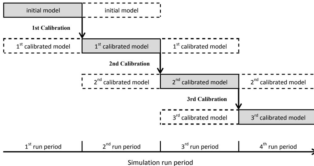
Figure 2 The process of recurrent calibration
