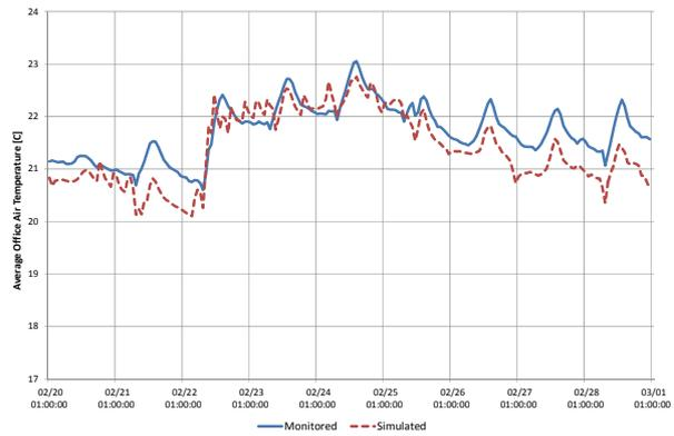
Figure 2 Monitored & simulated office temperature in 1<sup>st</sup> period: initial model (left), 1<sup>st</sup> calibrated model (right)
