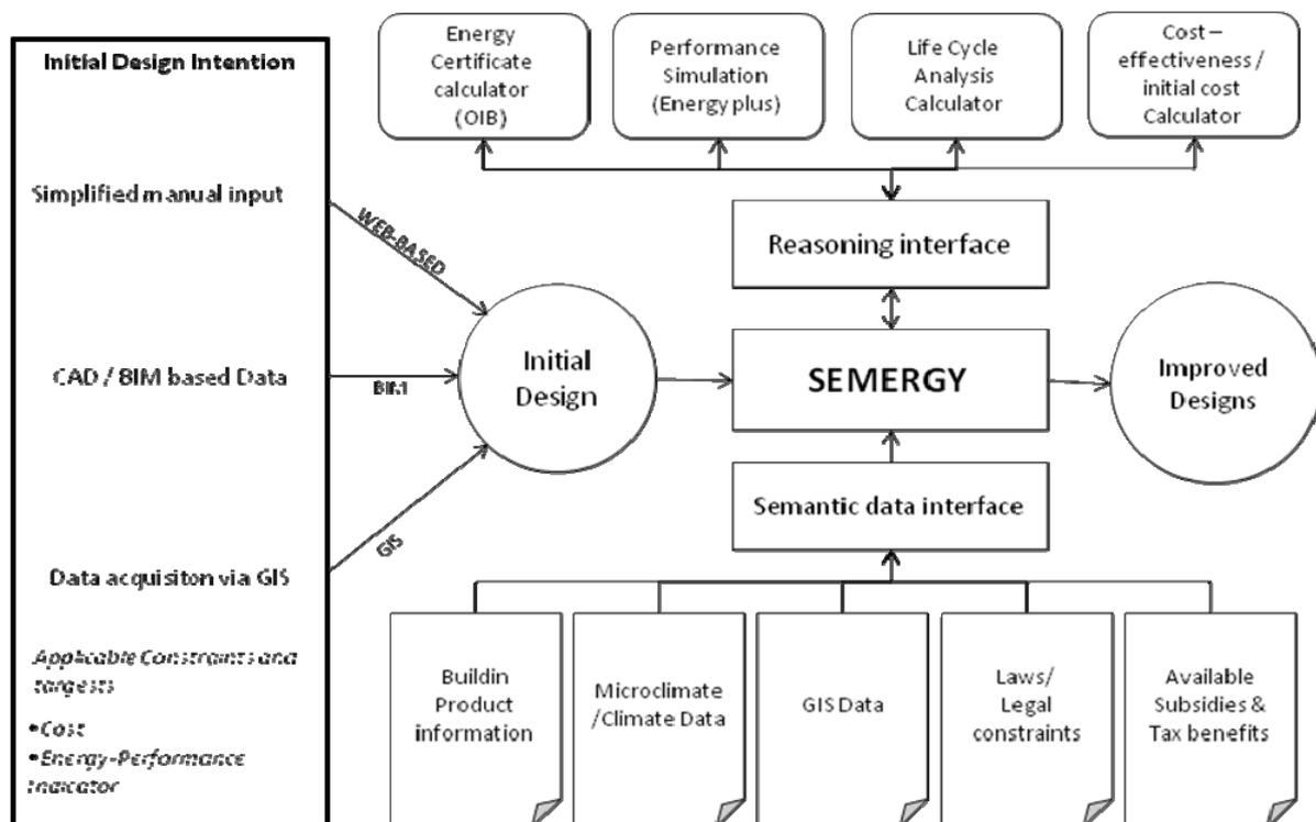
Figure 1 The general design of the SEMERGY environment
