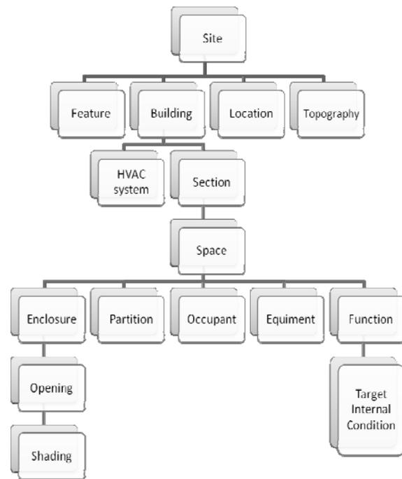
Figure 2 Building Data Model of SEMERGY (SBM)
