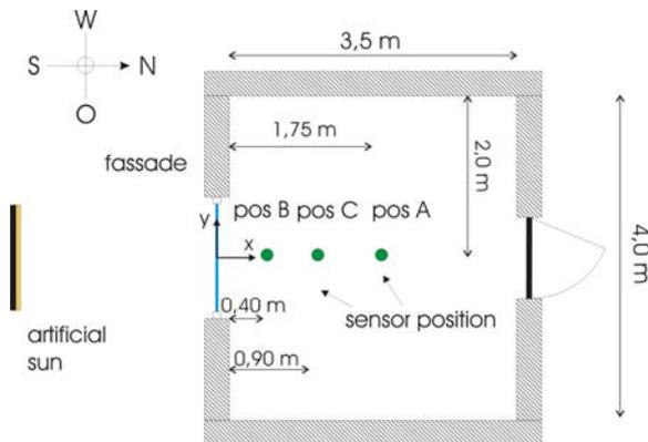
**Figure 1:** Test facility: climatic chamber dimensions and set up for different measurements
