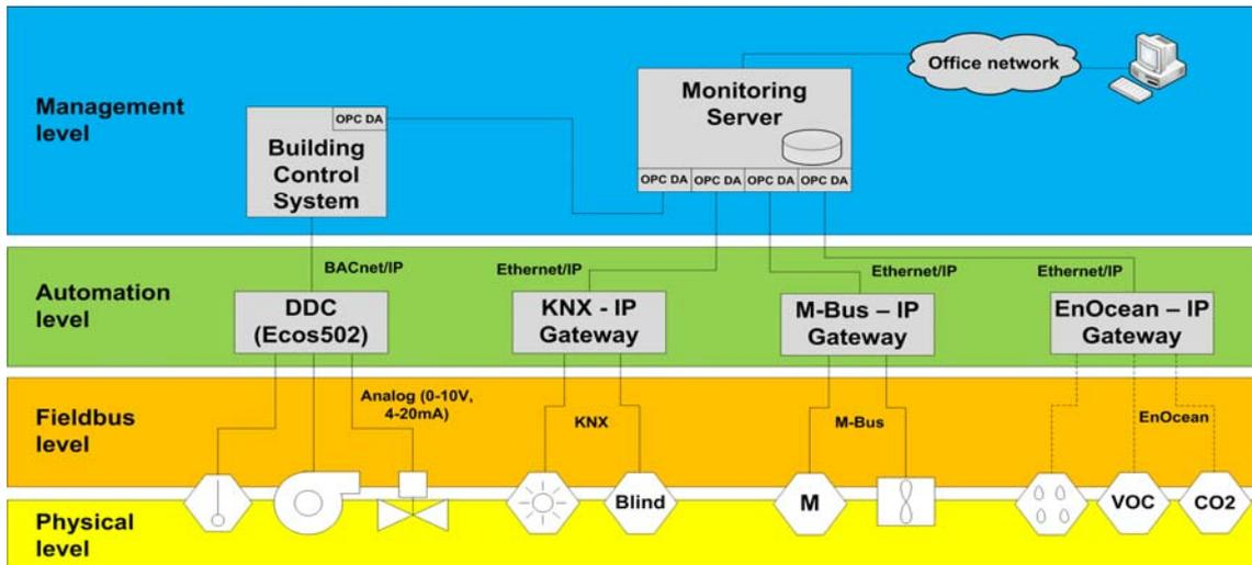
Figure 2 Four layer model of the monitoring system in Lehartrakt
