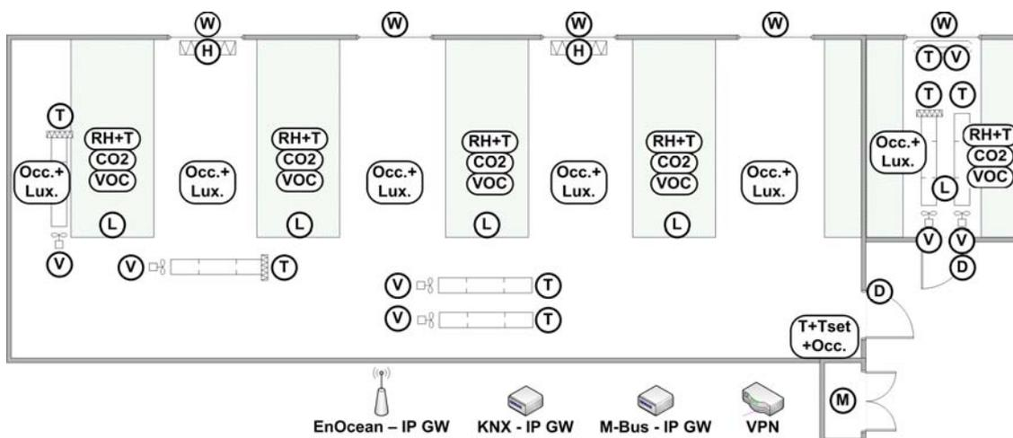
Figure 3 Floor plan including sensors of two laboratories in Lehartrakt
