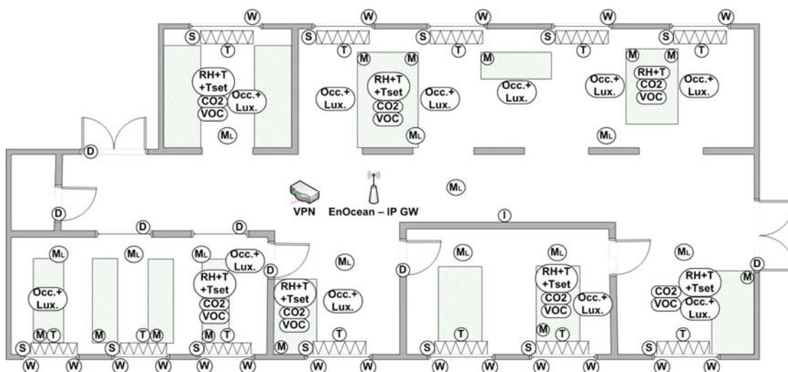
Figure 6 Floor plan including sensors in Karlsplatz
