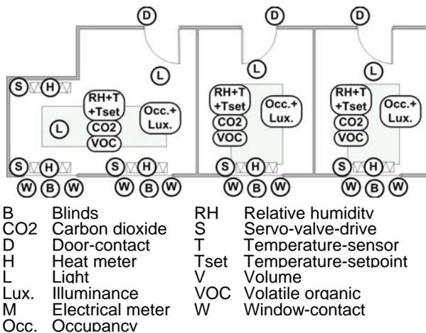
Figure 4 Floor plan including sensors of two office rooms and one conference room in Lehartrakt
