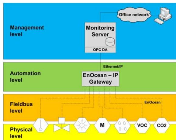
Figure 5 Four layer model of the monitoring system in Karlsplatz
