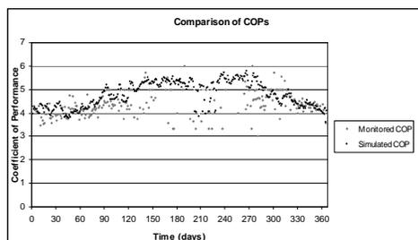
*Figure 2 Coefficient of performance of the heat pump obtained from monitored data compared with result of annual simulation*
