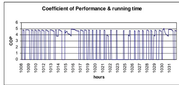
*Figure 3 Coefficient of performance of new heat pump in EnEV house in a typical winter day in February*
