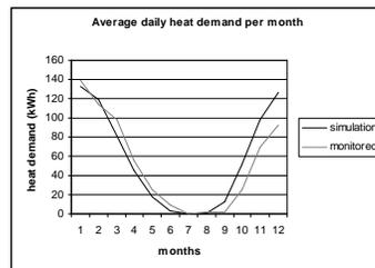
*Figure 1 A comparison of average monthly heat demand for space heating obtained from simulation with the results of annual monitoring*
