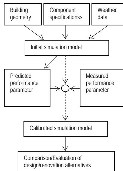
*Figure 12 Schematic illustration of simulation model generation, calibration, and application*
