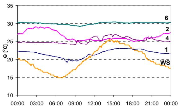
Figure 8 Measured outdoor (WS) and indoor temperature levels in hammam EC\_OP (04.03.2006). See Figure 5 for indoor sensor positions
