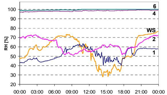
Figure 9 Outdoor (WS) and Indoor relative humidity levels in hammam EC\_OP (04.03.2006). See Figure 5 for indoor sensor positions
