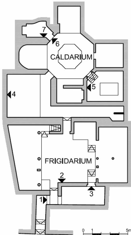
Figure 5 Schematic Cairo hammam plan with locations of the 7 internal data loggers (plan was generated based on a sketch by J. Bouillot)
