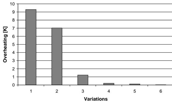
Figure 4 Overheating in building C (apartment, Vienna, overheating threshold=26°C). 1: base case without shading, ACH=1 h<sup>-1</sup>; 2: Similar to 1, with internal shades; 3: Similar to 1, with exterior shades; 4: Similar to 3, ACH=5 h<sup>-1</sup>; 5: Similar to 3, ACH=10 h<sup>-1</sup>; 6: Similar to 5 with PCM (25/26°C)
