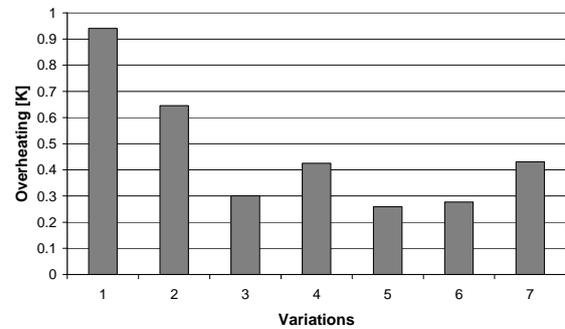
Figure 2 Overheating in building B (single house, Athens, overheating threshold=27°C). 1: base case without shading, ACH=1 h<sup>-1</sup>; 2: Similar to 1, with internal shades; 3: Similar to 1, with exterior shades; 4: Similar to 1 with fixed overhang; 5: Similar to 4, ACH=5 h<sup>-1</sup>; 6: Similar to 4, ACH=10 h<sup>-1</sup>; 7: Similar to 6 with PCM (26/28°C)
