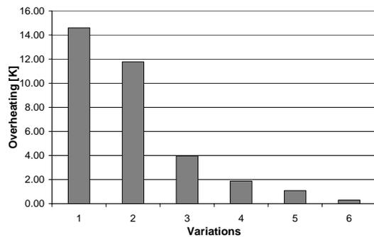
Figure 3 Overheating in building C (office use, Vienna, overheating threshold=26°C). 1: base case without shading, ACH=1 h<sup>-1</sup>; 2: Similar to 1, with internal shades; 3: Similar to 1, with exterior shades; 4: Similar to 3, ACH=5 h<sup>-1</sup>; 5: Similar to 3, ACH=10 h<sup>-1</sup>; 6: Similar to 5 with PCM (25/26°C)
