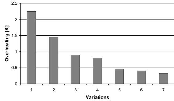
Figure 1 Overheating in building A (apartment, Athens, overheating threshold=27°C). 1: base case without shading, ACH=1h<sup>-1</sup>; 2: Similar to 1, with internal shades; 3: Similar to 1, with exterior shades; 4: Similar to 1 with fixed overhang; 5: Similar to 4, ACH=5h<sup>-1</sup>; 6: Similar to 4, ACH=10 h<sup>-1</sup>; 7: Similar to 6 with PCM (26/28°C)
