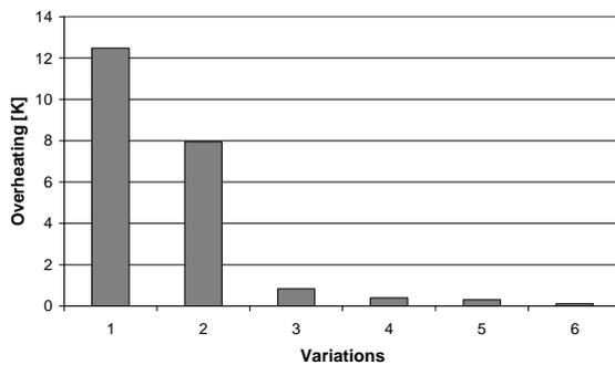
Figure 5 Overheating in building D (office use, Vienna, overheating threshold=26°C). 1: base case without shading, ACH=1 h<sup>-1</sup>; 2: Similar to 1, with internal shades; 3: Similar to 1, with exterior shades; 4: Similar to 3, ACH=5 h<sup>-1</sup>; 5: Similar to 3, ACH=10 h<sup>-1</sup>; 6: Similar to 5 with PCM (25/26°C)
