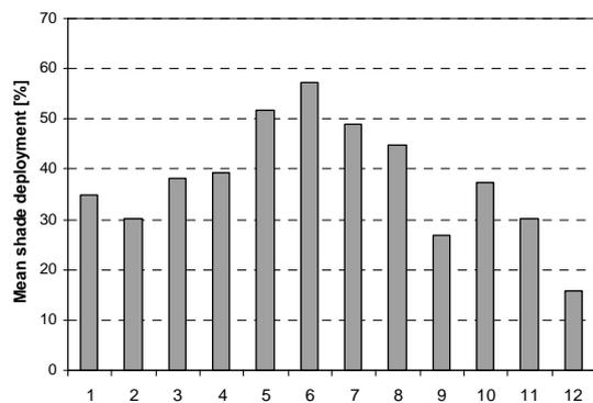
Figure 8 Mean shades deployment degree in FH\_TU (in %) over a period of one year (1: January; 12: December).
