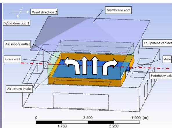
**Figure 4.** Structure of CASE-C (FSASR)
