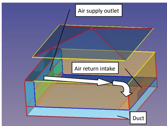
**Figure 3.** Structure of CASE-B (SSOR)
