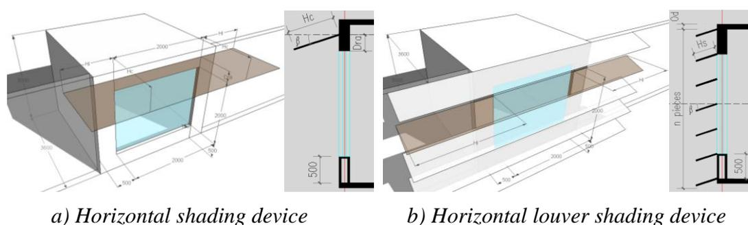
**Figure 1.** Parameters of Parametric geometry model (Unit: mm)
