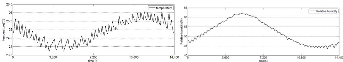
**Figure 7.** Temperature and humidity simulation results of valve duty ratio fuzzy control logic
