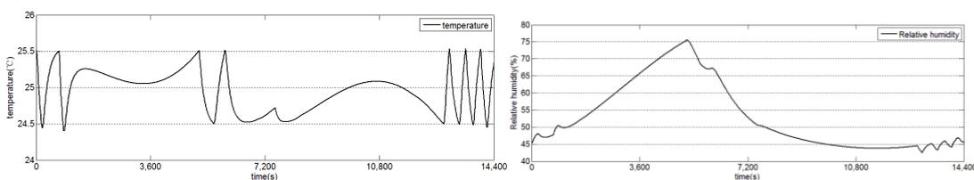
**Figure 6.** Temperature and humidity simulation results of conventional valve on/off control logic.
