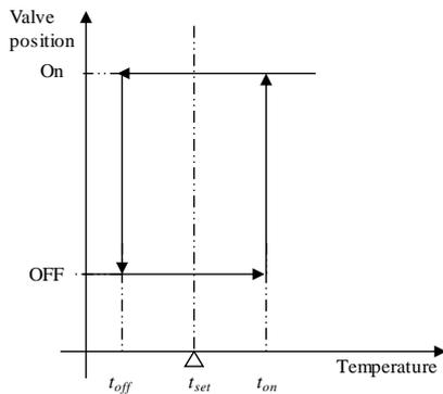
**Figure 4.** Conventional valve on/off control logic
