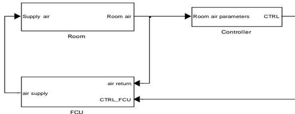
**Figure 1.** Simulation model built in the Matlab Simulink environment.
