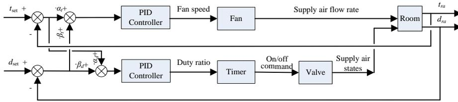
**Figure 3.** Flow chart of the newly proposed control logic
