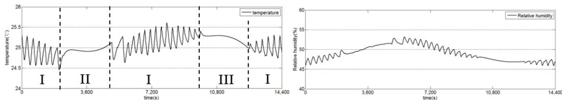
**Figure 5.** Temperature and humidity simulation results of proposed control logic
