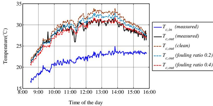
**Figure 4.** Comparison of calculated collector outlet temperatures with measured values for solar air collector with smooth airflow channel
