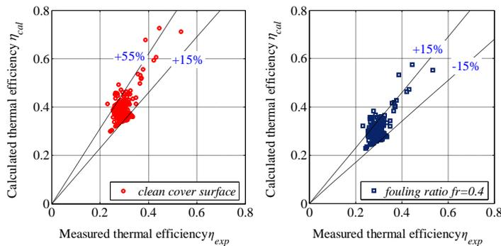
**Figure 8.** Relative error analysis of instantaneous thermal efficiencies with clean and fouling cover surfaces  $fr = 0.4$  for the collector with rectangular fin structure
