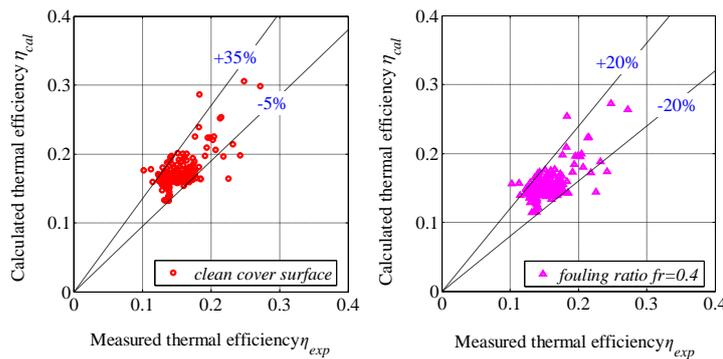
**Figure 5.** Relative error analysis of instantaneous thermal efficiencies with clean and fouling cover surfaces  $fr = 0.4$  for the collector with smooth airflow channel
