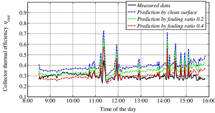
**Figure 6.** Comparison of calculated collector thermal efficiencies with measured values for solar air collector with rectangular fin structure
