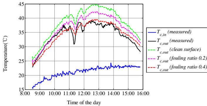
**Figure 7.** Comparison of calculated collector outlet temperatures with measured values for solar air collector with rectangular fin structure
