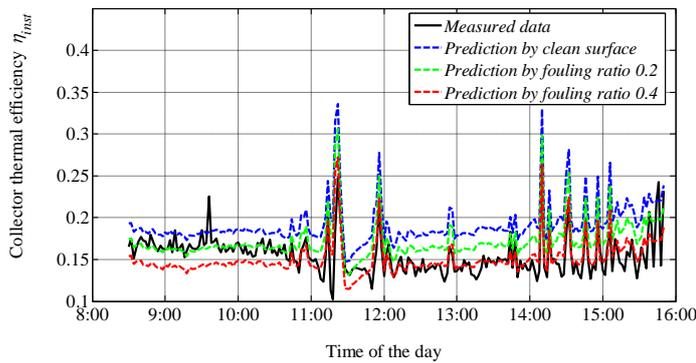
**Figure 3.** Comparison of calculated collector thermal efficiencies with measured values for solar air collector with smooth airflow channel
