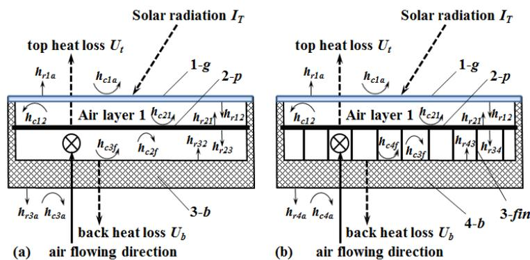
**Figure 1.** Cross-section schematic view of flat plate solar air collectors and heat transfer processes: (a) with smooth airflow channel; (b) with rectangular fin structure
