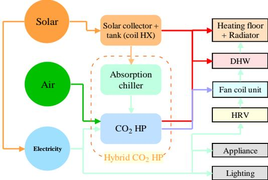
Figure 7. Design concept of energy system
