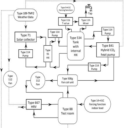
Figure 9. System layout in TRNSYS
