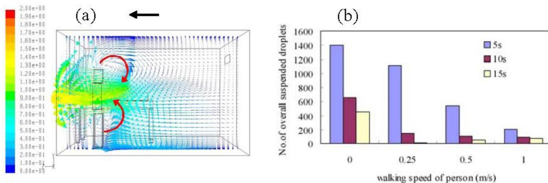
**Figure 4.** (a) Velocity vector distribution at  $x=3$  m at time= $2.5$  s and walking speed of  $1.0$  m/s
