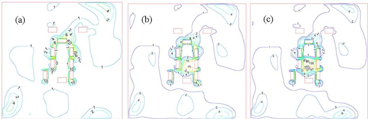
**Figure 5.** Concentration of BCPs (unit:  $\text{cfu/m}^3$ ) at  $z=1.1$  (a) when all surgical staff standing upright without movement (b) when surgeon 2 performing operation with  $45^\circ$  bending posture (c) at the end of bending back process
