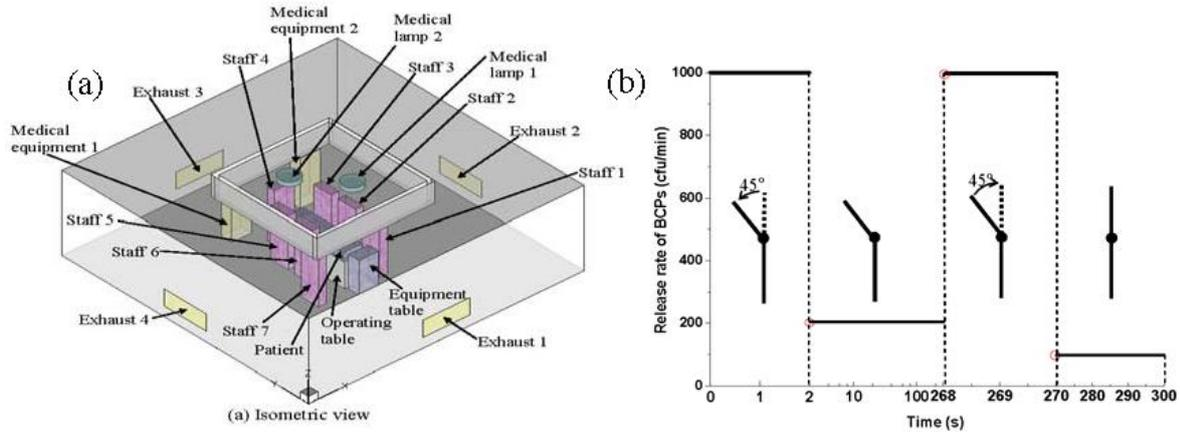
**Figure 2.** (a) Geometrical configuration of OT (b) Release rate of BCPs from staff 2 in a 5-minute bending cycle
