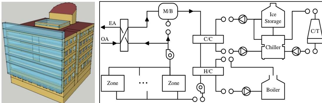
**Figure 2.** Whole building simulation modeling
