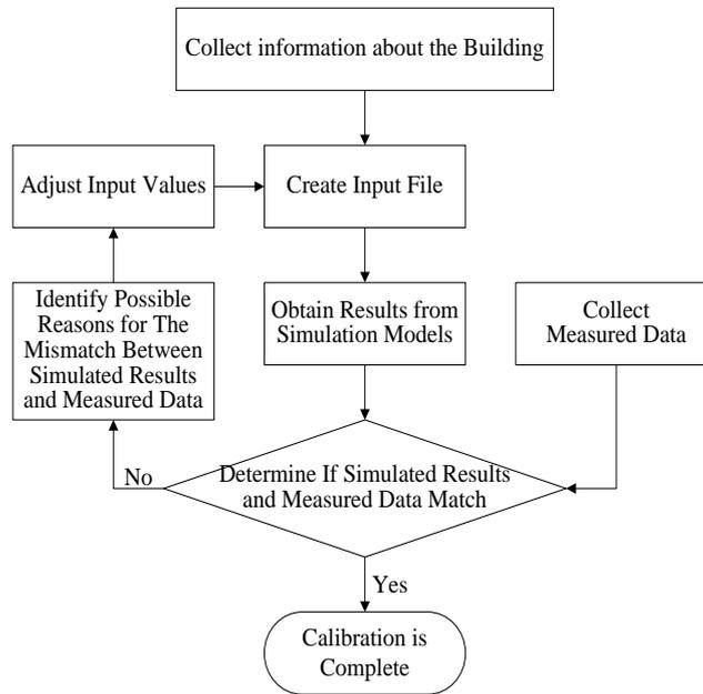
**Figure 1.** Calibration process of Model
