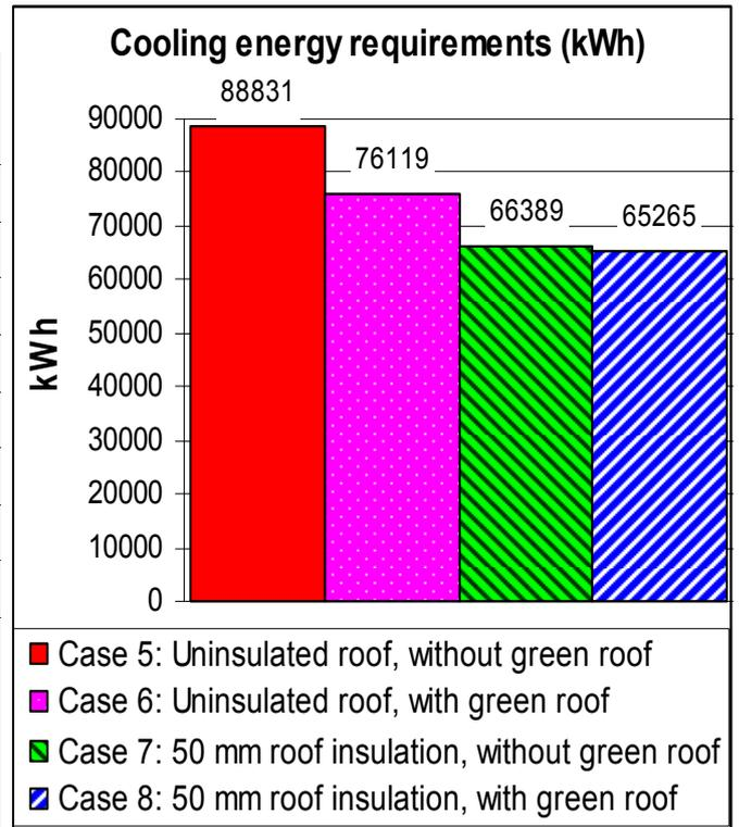
**Figure 6.** Heating (January) and cooling (July) energy requirements for the simulated cases
